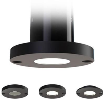
*\*Dimmable via MLV transformer & dimmer (fixture load must be 25% of MLV transformer max).*
