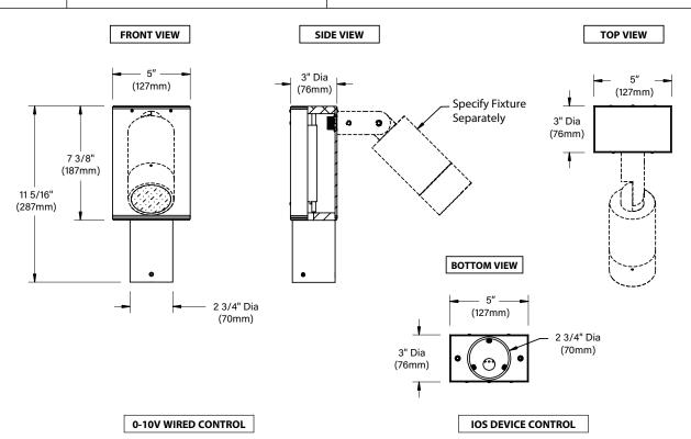
For use with: **C22** - 20WLED/1650-8000K + Dimming and CCT only (0-10V Wired Installation)
