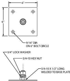
**YSF – Yoke Mount (YM) with Slipfitter**
