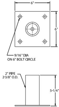
**KWA – Knuckle Slipfitter (KSF) with Wall Pole Mounting Arm**
