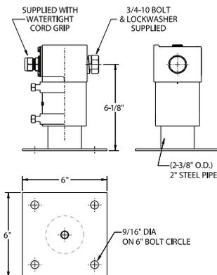
**YSWA – Yoke Mount (YM) with Slipfitter and Wall Pole Mounting Arm**
