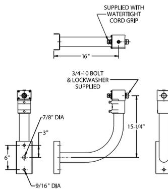
**YWB – Yoke Mount (YM) with Wall Bracket**
