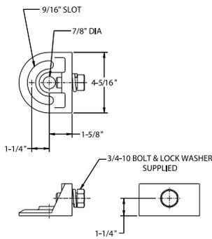
**YMS – Yoke Mount (YM) with Mounting Stud**
