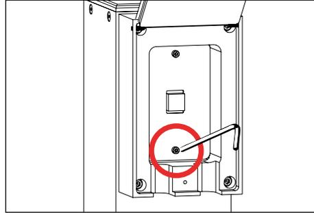
2. Loosen two (2) #6-32 screws with a 7/64" allen wrench to remove inner bracket with RJ45 jack.
