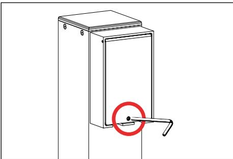
4. Receptacle cover has captive #6-32 screw. Secure receptacle by tightening captive #6-32 set screw using a 7/64" allen wrench.
