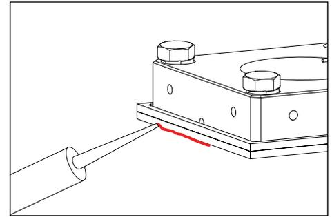
7. Mount base and plate to concrete using mounting holes drilled previously (mounting hardware not included). Minimum 1/4" diameter sleeve or wedge anchors for concrete must be used.
