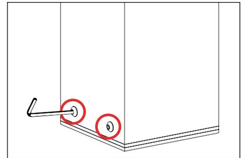
2. Attach ground from branch circuit to screw on anchor base. Place connectors inside receptacle.
