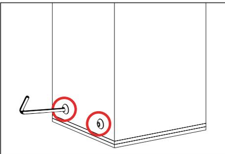
6. Attach in-use receptacle to installed anchor base and plate with four (4) #10-32 button head stainless steel cap screws at the base using a 1/8" allen wrench.
