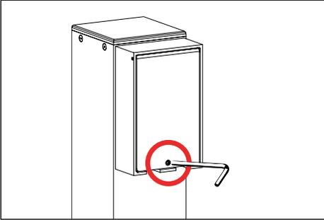
1. Open receptacle cover. Receptacle cover has captive #6-32 screw for use with a 7/64" allen wrench.
