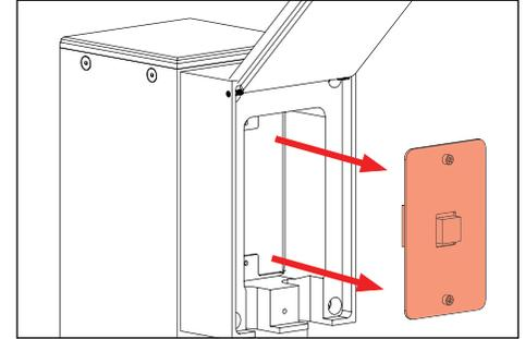
3. Connect incoming data cable to RJ45 jack as per installation plan. Follow manufacturer's instructions as per cable and method of connection to RJ45 jack (cable and connections required By Others). **See wiring diagram.**
