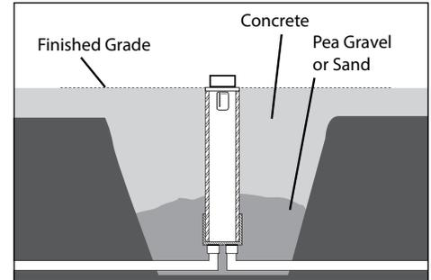
1. Excavate trench according to designed lighting plan. Dig hole a minimum of 24" deep and 10" wide to accommodate PVC housing at desired fixture location and direction of in-use receptacle(s).
