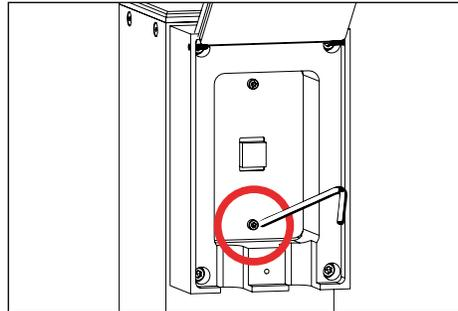
4. Place connections into bollard. Attach inner bracket with RJ45 jack with two (2) #6-32 screws with a 7/64" allen wrench.
