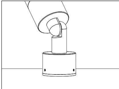
7. Insert fixture according to desired lighting plan.
