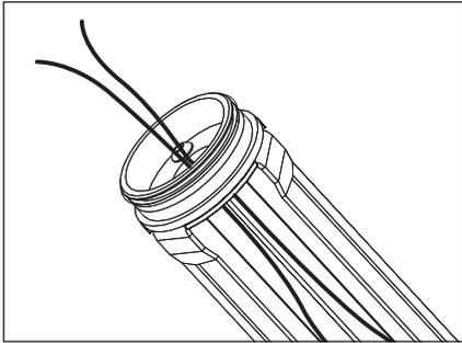
3. Pull low voltage wiring from remote 12V transformer (By Others) through the center of the anchor base and stake assembly.
