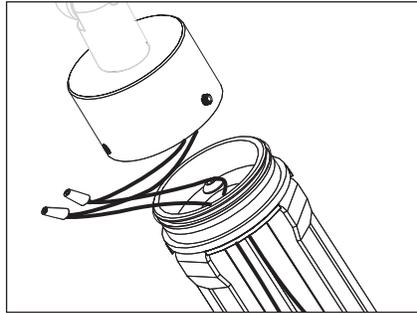
4. Make two connections from remote 12V transformer to fixture source leads using proper wire connectors (By Others). See wiring diagram.
