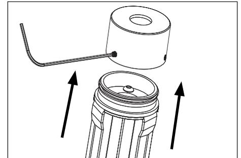
1. Use 5/64" Allen wrench loosen three (3) #8-32 stainless steel set screws (do not remove set screws from canopy). Remove canopy from stake.
