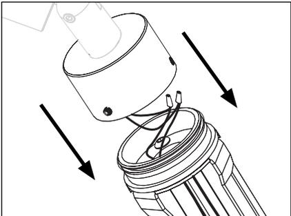
5. Place canopy onto stake and press firmly until the two pieces are fully seated.
