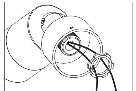
2. Mount fixture onto canopy by securing 1/2" NPS stem with provided locknut.
