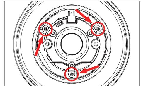
3. Use a .050" allen wrench to loosen three (3) set screws holding LED module. Gently lift from fixture.
