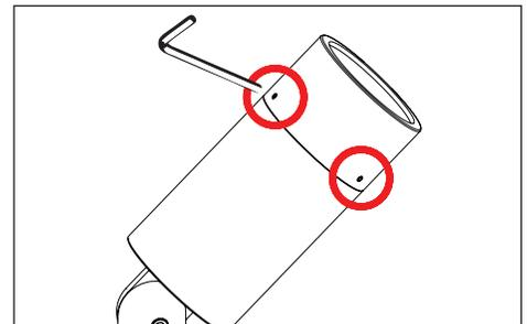
6. Place cap on fixture and tighten set screws until they are flush with the cap.
