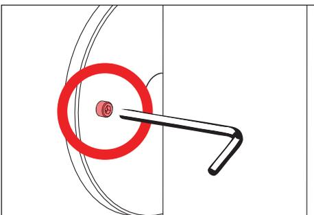
3. Mount fixture using two (2) #10-24 hex screws to installed back box. **Seal building envelope as per NEC. Do not overtighten.**
