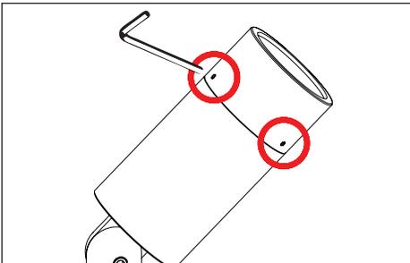
1. Use a 5/64" allen wrench to slightly loosen three (3) #8-32 stainless steel set screws to remove cap.
