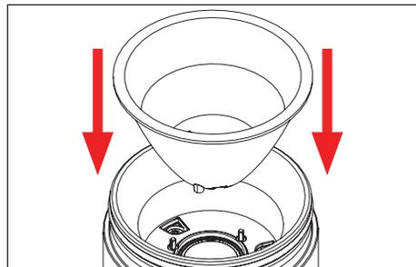
5. Replace optic by lining tabs with optic holder, then pressing down gently until secured into place.
