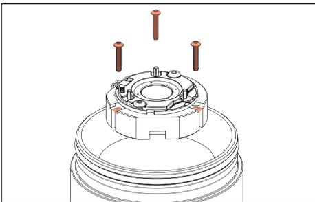
4. Gently lift LED module and disconnect from fixture. Install new LED module. Secure set screws using a .050" allen wrench.
