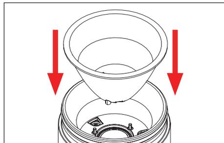
5. Replace optic by lining notches with optic holder, then pressing down gently until secured into place.
