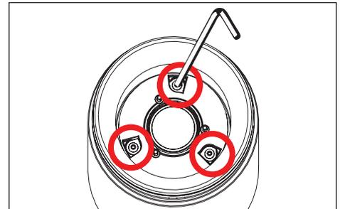
3. Use a .050" allen wrench to loosen three (3) set screws holding optic holder and LED module.
