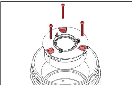
4. Gently lift LED module and disconnect from fixture. Install new LED module. Secure set screws through LED module and optic holder using a .050" allen wrench.
