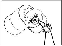
Mount knuckle onto canopy by securing 1/2" NPS stem with provided locknut.
