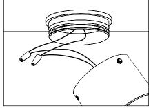
Make two connections from remote 12V transformer to fixture source leads using proper wire connectors (By Others). See wiring diagram.
