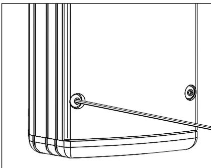
10. Make sure UPM housing gasket is free of any dirt or debris. Attach the faceplate by tightening the (4) #6-32 captive screws evenly using a 5/64" Allen wrench.
