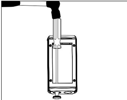
1. Remove faceplate, then remove Patented Knockout(s) as necessary from the inside of the UPM housing for branch circuit wiring and remote fixture leads. Leave remaining unused knockouts in place to maintain seal.
