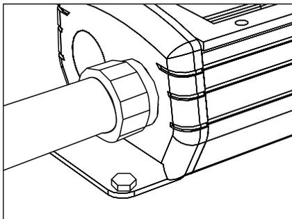
5. Connect 1/2" conduit connector through female threaded conduit entry.
