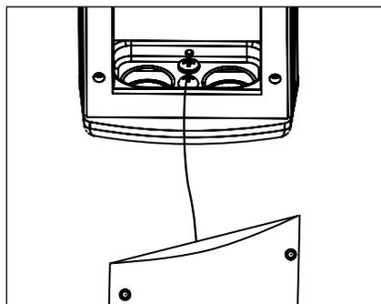
8. Attach tether wire under screw head at the base of the UPM housing. Slowly lower the faceplate until tether is taut.
