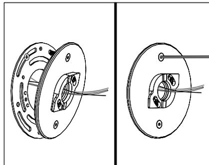
4. Feed branch circuit wiring and lamp leads to remote mounted fixture through mounting plate with CamLock™ assembly. Attach mounting plate with supplied (2) #10-24 stainless steel hex drive fasteners to universal ring using 1/8" Allen wrench.
