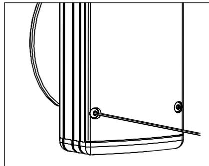
11. Make sure UPM housing gasket is free of any dirt or debris. Attach the faceplate by tightening the (4) #6-32 captive screws evenly to 6-9 in-lbs using a 5/64" Allen wrench.
