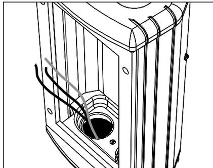
5. Pull branch circuit wiring necessary for installation (By Others.)
