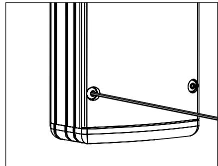
9. Make sure UPM housing gasket is free of any dirt or debris. Attach the faceplate by tightening the (4) #6-32 captive screws evenly using a 5/64" Allen wrench.
