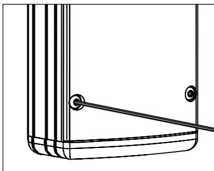
10. Make sure UPM housing gasket is free of any dirt or debris. Attach the faceplate by tightening the (4) #6-32 captive screws evenly using a 5/64" Allen wrench.
