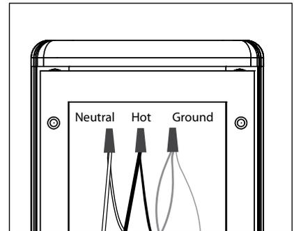
8. Use waterproof wire connectors (By Others) to connect driver primary leads to branch circuit wires. Connect incoming ground and driver ground to ground wire provided in UPM housing. **See wiring diagram.**
