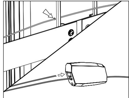
3. **Optional Step on PM2:** Thread safety cable through hole on the back of the UPM housing. Feed safety cable through opposing ends of the connector. Pull on wires to assure the connection is secure. Leave enough slack in safety cable for tree growth. Adjustments can be made by pressing release spring with a pin or 3/64" Allen tool.
