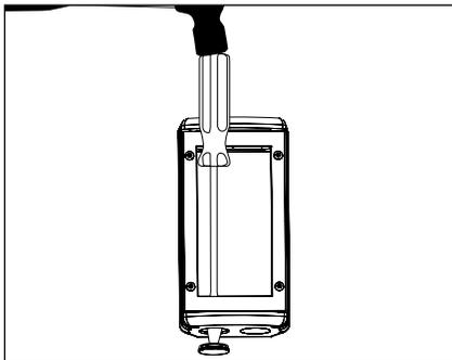
3. Remove Patented Knockout(s) as necessary from the inside of the UPM housing for branch circuit wiring and fixture leads to remote mounted fixture. Leave remaining unused knockouts in place to maintain seal.
