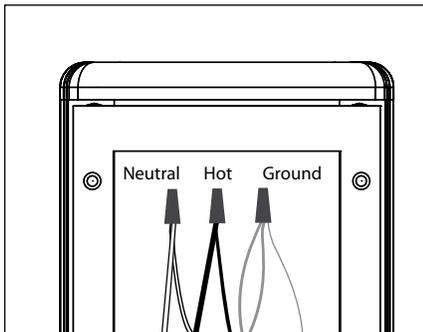
7. Use waterproof wire connectors (By Others) to connect driver primary leads to branch circuit wires. Connect incoming ground and driver ground to ground wire provided in UPM housing. **See wiring diagram.**
