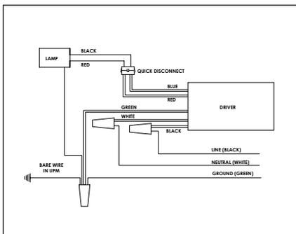
10. Pull lamp leads into UPM housing and connect to driver secondary leads using waterproof wire connectors (By Others).
