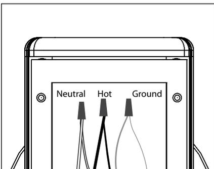
9. Use waterproof wire connectors (By Others) to connect driver primary leads to branch circuit wires. Connect incoming ground and driver ground to ground wire provided in UPM housing. See wiring diagram.
