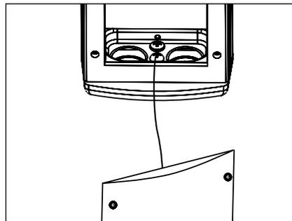
7. Attach tether wire under screw head at the base of the UPM housing and tighten. Slowly lower the faceplate until tether is taut.
