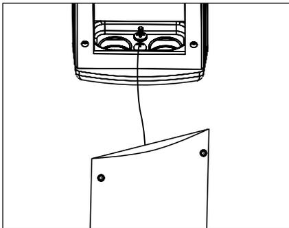
7. Attach tether wire under screw head at the base of the UPM housing and tighten. Slowly lower the faceplate until tether is taut.
