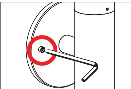
3. Using a 5/32" allen wrench mount fixture using two (2) #10-24 screws to installed back box. **Seal building envelope as per NEC. Do not overtighten.**
