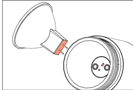
2. Firmly insert lamp pins into socket to make connection. Rocking motion may be required.
