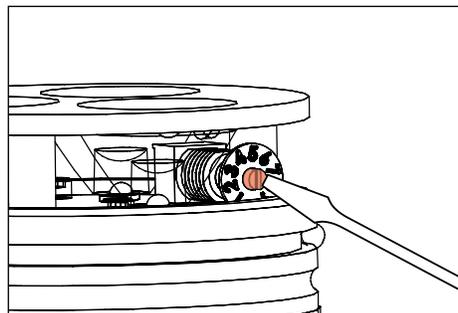
2. With flat head screw driver rotate dial to desired lumen output.
