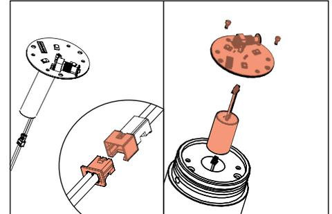
4. Disengage LED board and driver assembly. Replace with new board and driver assembly.
