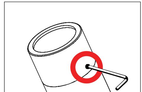
3. Place cap on fixture and tighten set screw. Tighten screw to 1/2 in-lbs. Top of screw should sit flush with fixture cap.
