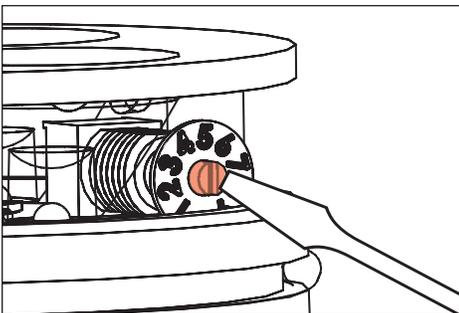
7. With flat head screw driver rotate dial to desired lumen output.
