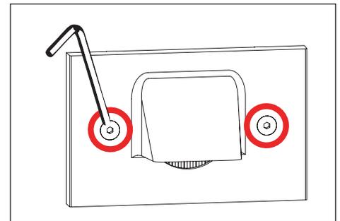
9. Mount faceplate using two (2) #10-24 screws with a 1/8" allen wrench. Tighten evenly to compress gasket. **Do not over tighten.**
