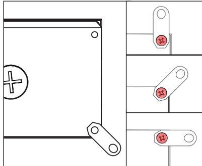
3. To prepare MB2 for mounting, align mounting brackets on back of box. Brackets can be aligned to vertical, horizontal or 45° orientation. Secure with mounting screw using screwdriver.
