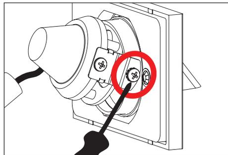
8. Attach bracket to faceplate by securing two (2) phillips screws. Aim to desired position. Tighten two (2) phillips screws to lock in place when desired angle is set.
