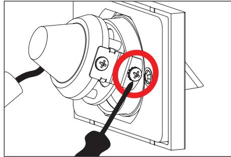
2. Loosen two (2) phillips head screws holding bracket to faceplate. Remove bracket from faceplate to expose optics and LED.
