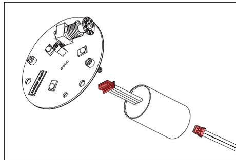
5. Disengage LED board and driver assembly. Replace with new board and driver assembly.
