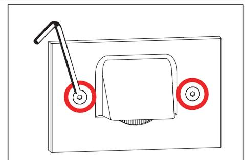
3. Mount faceplate using two (2) #10-24 screws with a 1/8" allen wrench. Tighten evenly to compress gasket. **Do not over tighten.**
