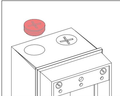
1. Remove canopy and/or fixture from MB2 housing. Ensure unused tapped holes are plugged to maintain seal. Plugs are included.
