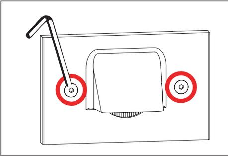
1. Remove fixture by loosening two (2) #10-24 fasteners. Gently pull away from installed back box enough to expose back of faceplate.
