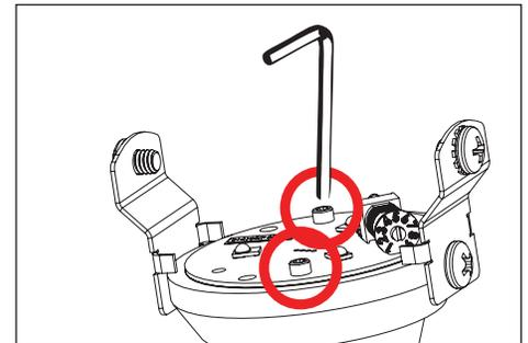
6. Reverse install LED board and driver by carefully re-engaging quick disconnects. Secure LED board in place with stainless steel screws. Snap optics in place.
