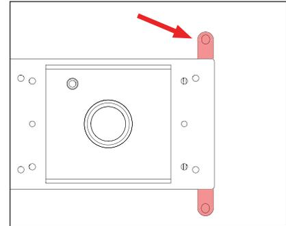
4. Mount MB2 box to surface using mounting hardware (included) using the mounting brackets attached to back of MB2 box.
