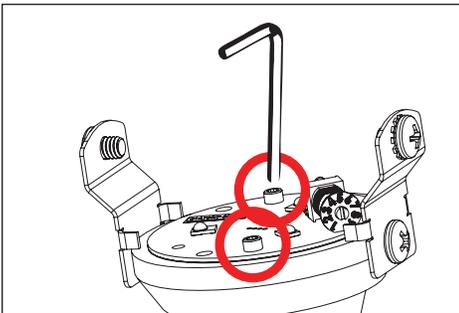
4. Use a 5/64" allen wrench to remove two (2) #2-56 socket head cap screws on LED board, grasp LED board and gently pull up to expose quick disconnect.
