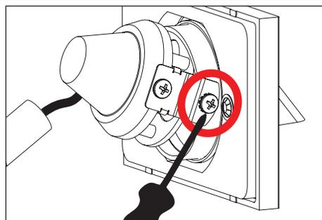
2. To aim, loosen the two (2) phillips screws attaching the adjustable bracket to the faceplate. Aim to desired position. Tighten two (2) phillips screws to lock in place when desired angle is set.
