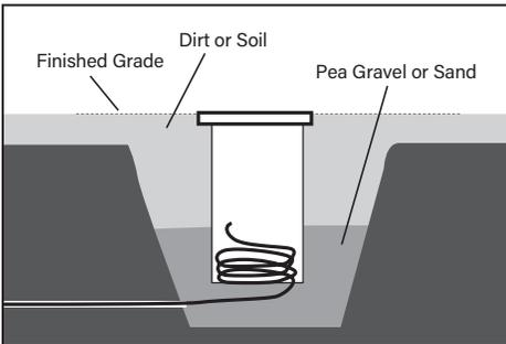
5. Align and orientate concrete pour collar on housing to illuminated object. Back fill with pea gravel or sand to allow sufficient drainage. Install housing flush at grade. **See wiring diagram.**
