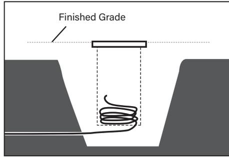
2. Supply low voltage wiring necessary for installation.
