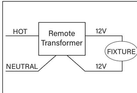
6. Make watertight connections from remote transformer to fixture leads using waterproof wire connectors (not included).
