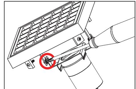
7. Loosen stainless steel phillips head cap screw on adjustable bracket, aim to desired location. Tighten to maintain aiming position.
