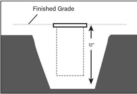
1. Excavate trench according to designed lighting plan 20" deep and 10" wide suitable for the 13" fixture housing.
