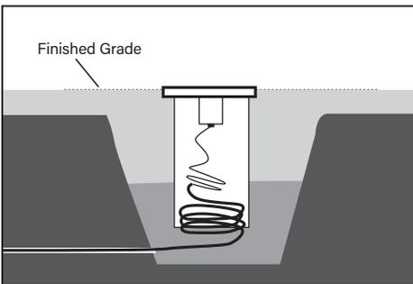
8. Attach faceplate to concrete pour collar with four (4) 1/4-20 screws using a 3/16" allen wrench.
