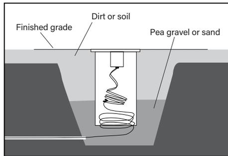
5. Back fill with pea gravel or sand to allow sufficient drainage. Install housing flush at grade. Install faceplate with two (2) 1/4-20 screws using a 3/16" allen wrench.
