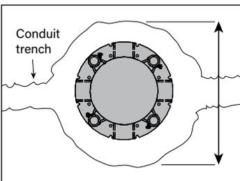
B. Excavate a hole to the necessary dimensions for fixture placement according to lighting plan.
