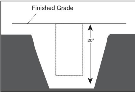
1. Excavate trench according to designed lighting plan, 20" deep and 10" wide suitable for the 13" fixture housing.
