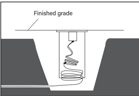
4. Insert fixture housing and low voltage wire into trench.
