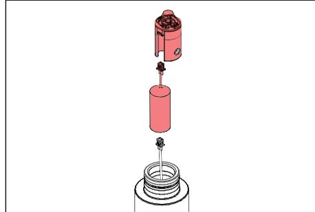
2. For BKSSL: Pull the heat sink from the body to expose the LED board and Driver components. Utilize quick disconnects to change modular LED and driver components. Re-install the heat sink into body.
