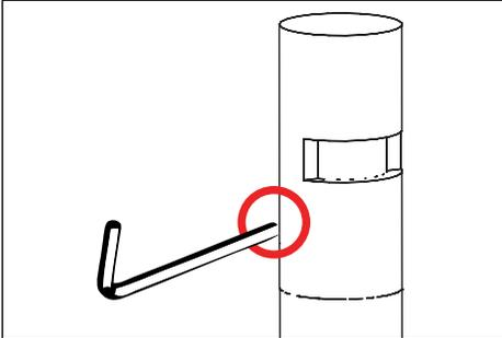
1. Loosen #8-32 stainless steel set screw on cap using a 5/64" Allen wrench and remove.
