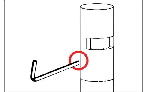
3. Place cap on fixture and tighten set screw. Tighten screw to 1/2 inch pounds. Top of screw should sit flush with fixture cap.
