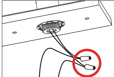
3. Make watertight connections from remote transformer to fixture leads using waterproof wire connectors. See wiring diagram.
