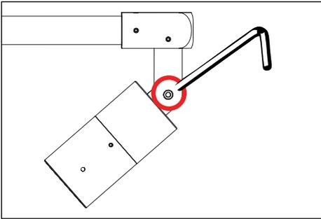
1. Use a 5/32" allen wrench to slightly loosen #10-32 stainless steel set screw on the stem for 180° aiming purpose.
