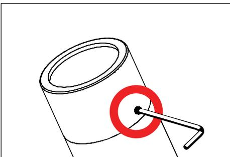
1. Use a 5/64" allen wrench to loosen #8-32 stainless set screw and remove cap.
