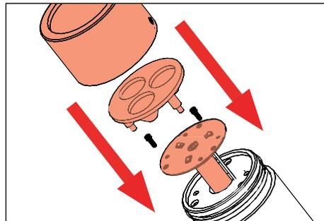
5. Reverse install LED board and driver by carefully wrapping 18 gauge wires around driver and inserting into fixture body. Secure LED board in place with stainless steel screws.
