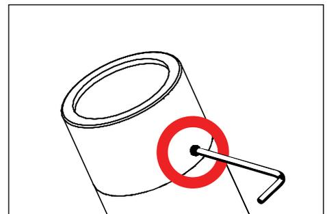
3. Place cap on fixture and tighten set screw. Tighten screw to 1/2 in-lbs. Top of screw should sit flush with fixture cap.
