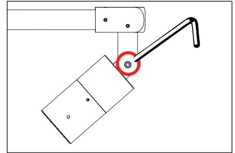
3. Tighten #10-32 stainless steel set screw using a 5/32" allen wrench to secure aiming position.
