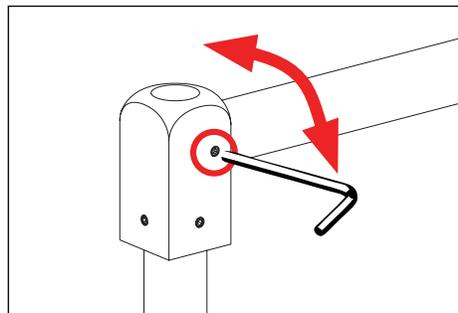
5. To adjust stem, loosen #8-32 screw with a 5/64" allen wrench at stem cap. Adjust as needed, then secure.
