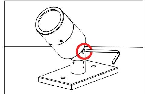
3. Use a 5/32" allen wrench to loosen #10-32 stainless steel black oxide socket head cap screw at the knuckle for vertical aiming purpose.
