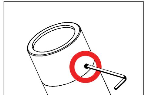
6. Place cap on fixture and tighten set screw. Tighten screw to 1/2 in-lbs. Top of screw should sit flush with fixture cap.
