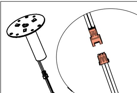
4. Disengage LED board and driver assembly. Replace with new board and driver assembly.
