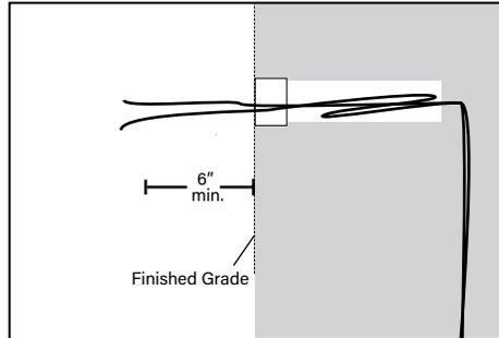
5. Supply low voltage wiring necessary for installation. Loop minimum of 6" of low voltage wire behind mounted collar to allow for fixture service.
