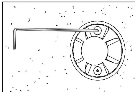
7. Mount faceplate to collar using two (2) #6-32 x 5/8" flat head cap screws (included) with a 5/64" allen wrench.
