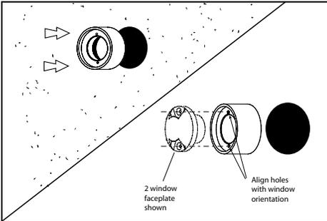
4. Fit flush mount collar into hole so it is flush with finished surface. Wipe off any excess adhesive.
