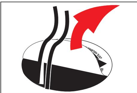
8. Remove temporary cover and pull out low voltage wire.
