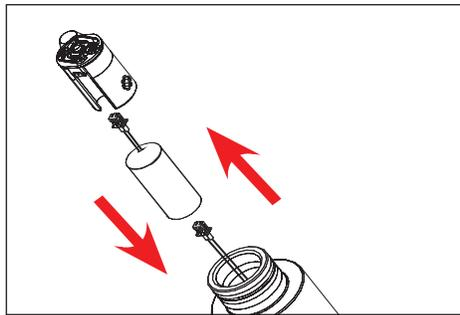
2. Pull the heat sink from the body to expose the LED board and Driver components. Utilize quick disconnects to change modular LED and driver components. Re-install the heat sink into body.
