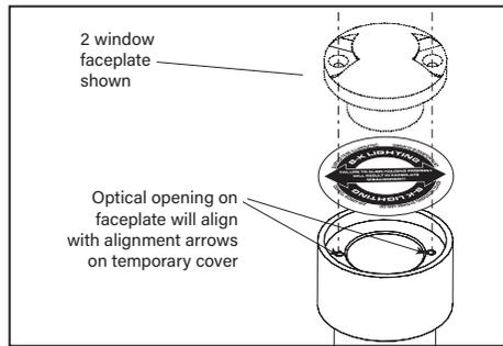
6. Align holes to final installation orientation. Point arrows on temporary cover toward surface to be illuminated.
