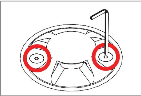
10. Mount faceplate to collar using two (2) #6-32x5/8" flat head screws (included) with a 5/64" allen wrench.
