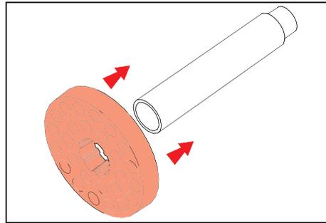
3. Slide stability flange onto power pipe.
