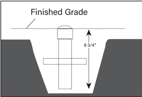
1. Excavate trench according to designed lighting plan 10" deep and 10" wide suitable for the 8-3/4" fixture housing. See Dig-It Guide at [www.bklighting.com/dig-it](http://www.bklighting.com/dig-it) for proper soil preparation information.
