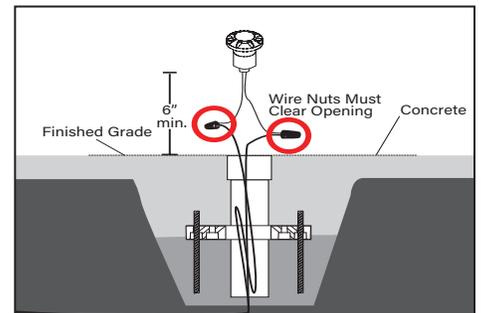
9. Access low voltage wire inside power pipe. Make watertight connections using waterproof wire connectors (not included). Wire connectors must clear opening. Insert fixture and low voltage wire into power pipe.
