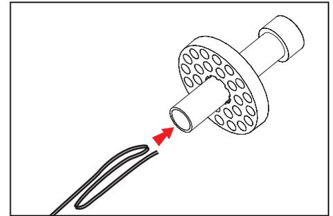
4. Loop minimum of 6" of low voltage wire inside power pipe to allow for fixture service.
