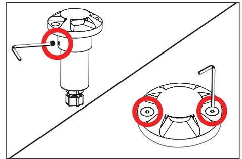
3. Replace faceplate assembly and tighten set screw. Re-Install fixture.
