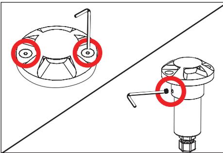
1. Loosen #8-32 set screw on faceplate assembly using a 5/64" allen wrench and remove. Loosen set screw on collar and remove.
