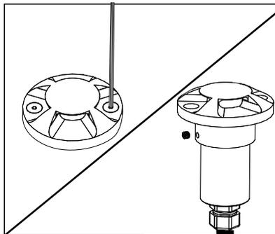
1. Loosen #8-32 set screw on faceplate assembly using a 5/64" Allen wrench and remove. Loosen set screw on collar and remove.
