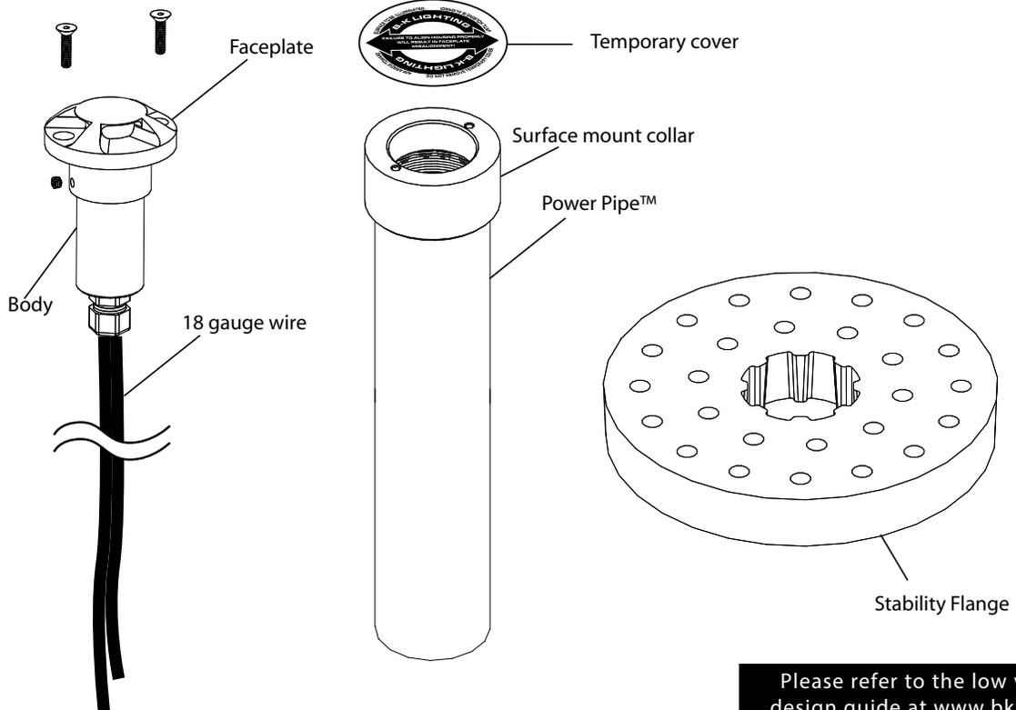
Please refer to the low voltage design guide at [www.bklighting.com/lvguide](http://www.bklighting.com/lvguide) before installation for proper wire selection.
