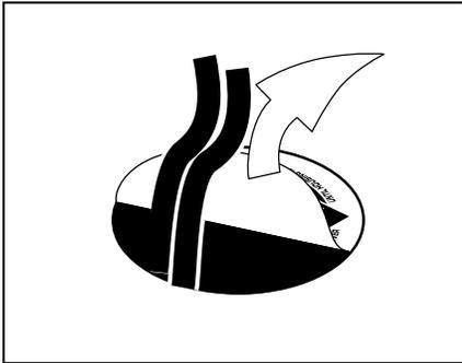
8. Remove temporary cover and pull out low voltage wire.
