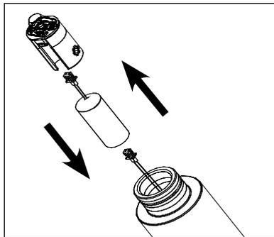
2. Pull the heat sink from the body to expose the LED board and Driver components. Utilize quick disconnects to change modular LED and driver components. Re-install the heat sink into body.
