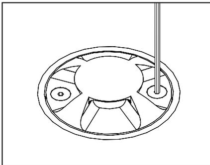
10. Mount faceplate to collar using (2) #6-32x5/8" flat head screws (provided) with a 5/64" Allen wrench.
