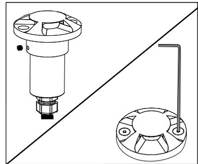
3. Replace faceplate assembly and tighten set screw. Re-Install fixture.
