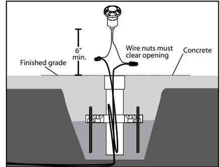
9. Access low voltage wire inside Power Pipe™. Make two watertight connections using waterproof wire connectors (By Others). Wire nuts must clear opening. Insert fixture and low voltage wire into Power Pipe™.
