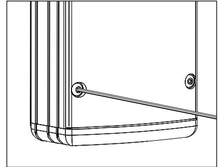
9. Make sure UPM body gasket is free of any dirt or debris. Attach the faceplate by tightening the (4) #6-32 captive screws evenly to 6-9 in/lbs using a 5/64" allen wrench.
