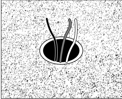
6. Pull branch circuit wiring necessary for installation (By Others).
