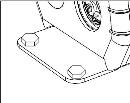
4. Attach the UPM housing at mounting brackets with 1/4" fasteners (by others). Use suitable mounting hardware for surface.
