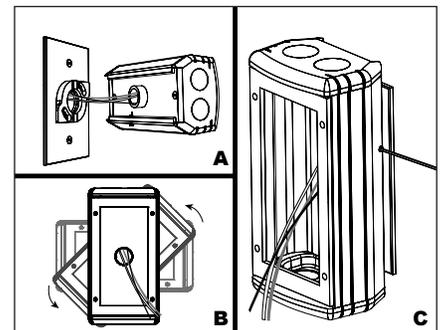
4. Feed wire into UPM housing. Install housing on CamLock™ at 90° to finished orientation as shown. (Figure A)
