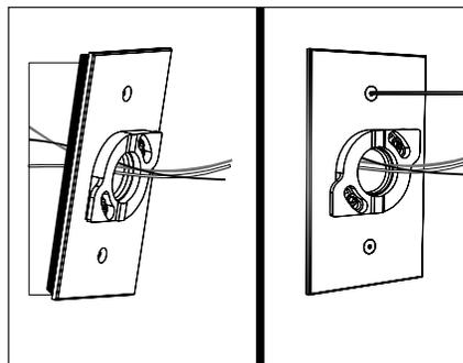
3. Feed branch circuit wiring through mounting plate with CamLock™ assembly. Attach mounting plate with supplied (2) #6-32 stainless steel hex drive fasteners to recessed junction box using a 5/64" allen wrench.
