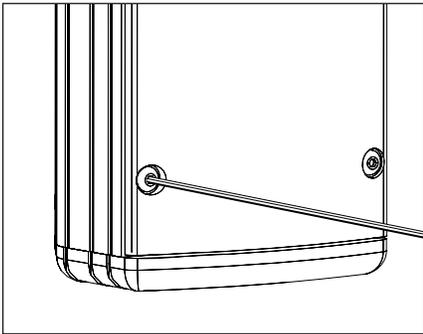
9. Make sure UPM body gasket is free of any dirt or debris. Attach the faceplate by tightening the (4) #6-32 captive screws evenly to 6-9 in/lbs using a 5/64" allen wrench.
