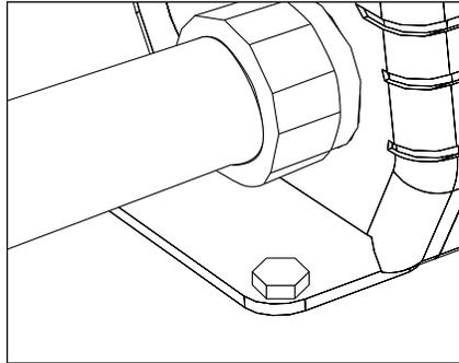
5. Connect 1/2" conduit connector through female threaded conduit entry.
