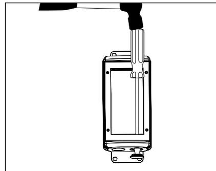
3. Remove Patented Knockout(s) as necessary from the inside of the UPM housing. Leave remaining unused knockouts in place to maintain seal.
