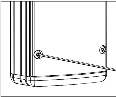
8. Make sure UPM body gasket is free of any dirt or debris. Attach the faceplate by tightening the (4) #6-32 captive screws evenly to 6-9 in/lbs using a 5/64" allen wrench.
