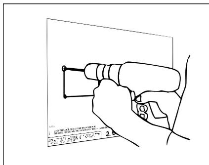
2. Drill holes into surface for 1/4" fasteners (by others) on locations illustrated on template.
