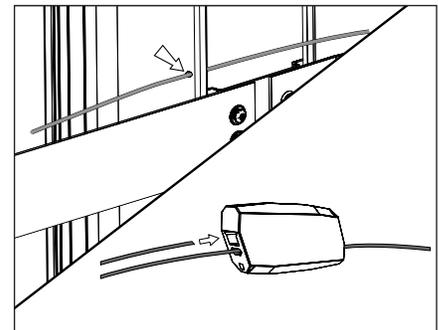
**Optional Step on PM1 & PM2:** Thread safety cable through hole on the back of the UPM housing. Feed safety cable through opposing ends of the connector. Pull on wires to assure the connection is secure. Leave enough slack in safety cable for tree growth. Adjustments can be made by pressing release spring with a pin or 3/64" allen tool.
