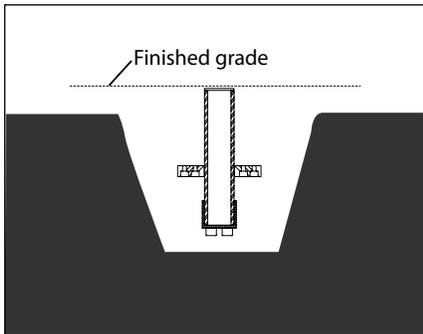
1. Excavate trench according to designed lighting plan. Dig hole a minimum of 24" deep and 10" wide to accommodate PowerPipe™ at desired fixture locations.
