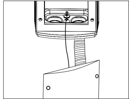
6. Attach tether wire under screw head at the base of the UPM housing and tighten. Slowly lower the faceplate until tether is taut.
