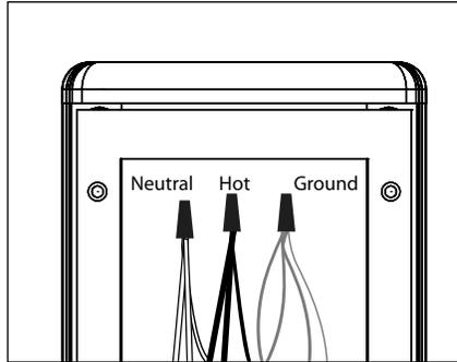
8. Use wire connectors (By Others) to connect branch circuit leads to lamp leads. Connect incoming ground and lamp ground to ground wire provided in UPM housing.
