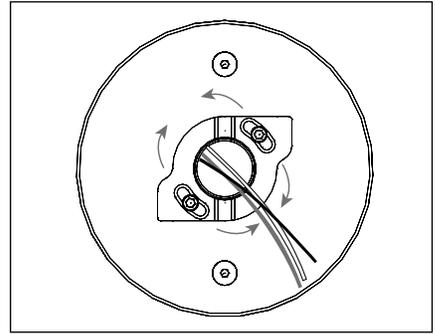
4. Feed branch circuit wiring through mounting plate with CamLock™ assembly. Attach mounting plate with supplied (2) #10-24 stainless steel hex drive fasteners to universal ring using 1/8" allen wrench.
