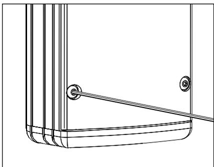
10. Make sure UPM body gasket is free of any dirt or debris. Attach the faceplate by tightening the (4) #6-32 captive screws evenly to 6-9 in/lbs using a 5/64" allen wrench.
