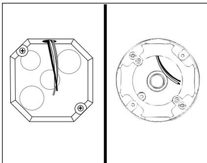
1. Install standard 4" octagonal/round recessed junction box in the final fixture location according to designed lighting plan.
