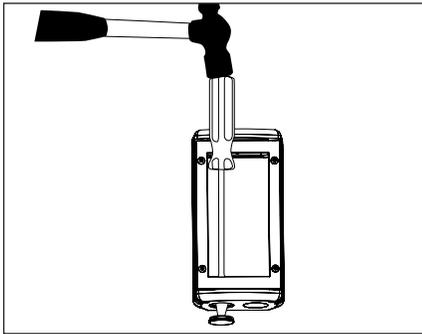
1. Remove Patented Knockout(s) as necessary from the inside of the UPM housing for branch circuit wiring and lamp leads to remote mounted fixture. Leave remaining unused knockouts in place to maintain seal.
