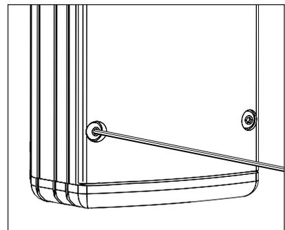
9. Make sure UPM body gasket is free of any dirt or debris. Attach the faceplate by tightening the (4) #6-32 captive screws evenly to 6-9 in/lbs using a 5/64" allen wrench.
