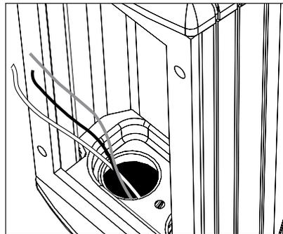
5. Pull branch circuit wiring necessary for installation (By Others.)
