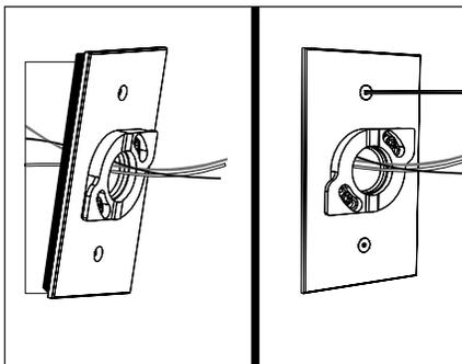
3. Feed branch circuit wiring and lamp leads to remote mounted fixture through mounting plate with CamLock™ assembly. Attach mounting plate with supplied (2) #6-32 stainless steel hex drive fasteners to recessed junction box using a 5/64" allen wrench.
