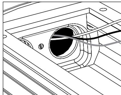
6. Pull branch circuit wiring necessary for installation (By Others.)
