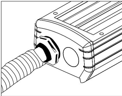
4. Connect 1/2" conduit connector through female threaded conduit entry.
