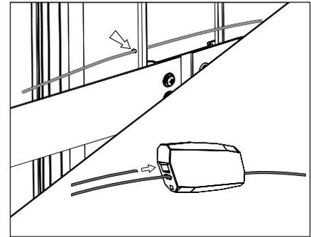
3. **Optional Step on PM1 & PM2:** Thread safety cable through hole on the back of the UPM housing. Feed safety cable through opposing ends of the connector. Pull on wires to assure the connection is secure. Leave enough slack in safety cable for tree growth. Adjustments can be made by pressing release spring with a pin or 3/64" allen tool.
