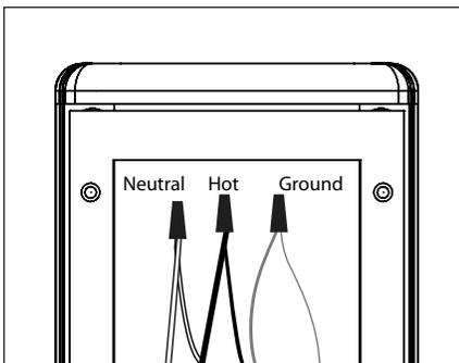
7. Use wire connectors (By Others) to connect transformer primary leads to branch circuit wires. Connect incoming ground to ground wire provided in UPM housing. See wiring diagram.
