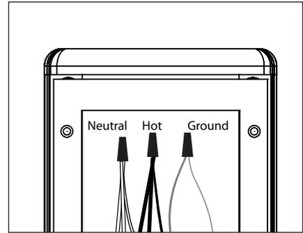
6. Use wire connectors (By Others) to connect both transformers primary leads to branch circuit wires. Connect incoming ground to ground wire provided in UPM housing. See wiring diagram.
