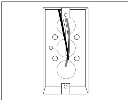
1. Install standard 4.5" x 2.85" recessed junction box (by others) in the final fixture location according to designed lighting plan.
