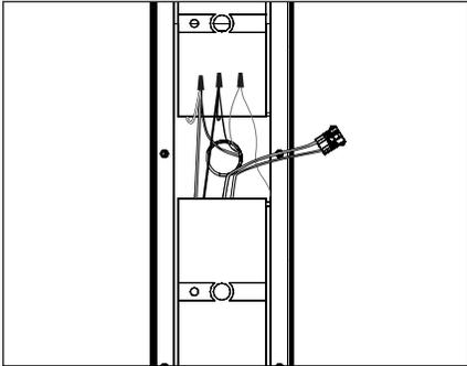
8. Remove the backing from adhesive tape on transformers, place in bottom of UPM housing void of any wiring and press firmly for five seconds to ensure good contact.
