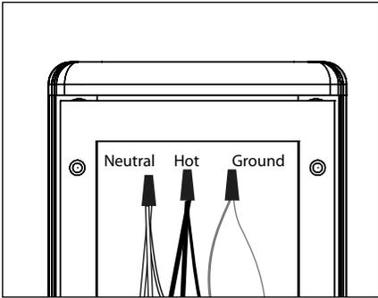
8. Use wire connectors (By Others) to connect both transformers primary leads to branch circuit wires. Connect incoming ground to ground wire provided in UPM housing. See wiring diagram.
