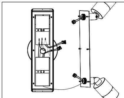
11. Connect transformers secondary leads to lamp leads using pre-wired factory connector.
