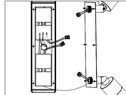
10. Connect transformers secondary leads to lamp leads using pre-wired factory connector.
