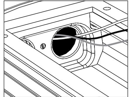
6. Pull branch circuit wiring necessary for installation (By Others.)
