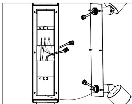
10. Connect transformers secondary leads to lamp leads using pre-wired factory connector.
