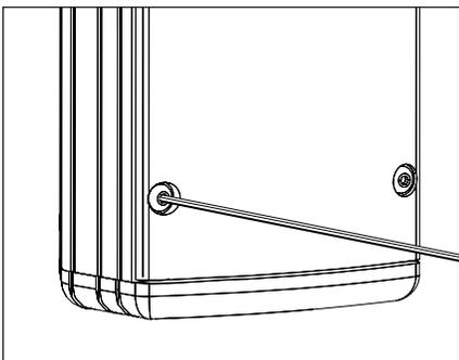
11. Make sure UPM body gasket is free of any dirt or debris. Attach the faceplate by tightening the (4) #6-32 captive screws evenly to 6-9 in/lbs using a 5/64" allen wrench.
