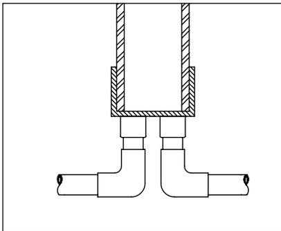
2. Connect conduit to the 1/2" conduit couplers attached to the bottom of the PowerPipe™. Place PowerPipe™ in hole.
