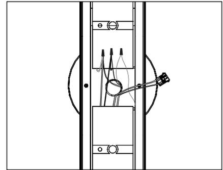
9. Remove the backing from adhesive tape on transformers, place in bottom of UPM housing void of any wiring and press firmly for five seconds to ensure good contact.
