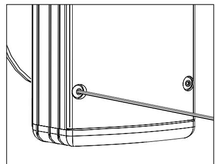
12. Make sure UPM body gasket is free of any dirt or debris. Attach the faceplate by tightening the (4) #6-32 captive screws evenly to 6-9 in/lbs using a 5/64" allen wrench.
