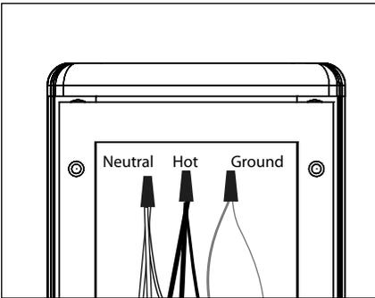
7. Use wire connectors (By Others) to connect both transformers primary leads to branch circuit wires. Connect incoming ground to ground wire provided in UPM housing. See wiring diagram.
