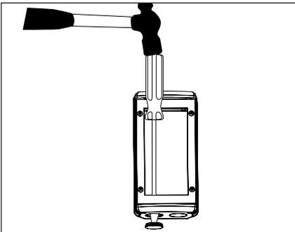
1. Remove Patented Knockout(s) as necessary from the inside of the UPM housing. Leave remaining unused knockouts in place to maintain seal.
