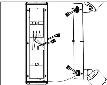
9. Connect transformers secondary leads to lamp leads using pre-wired factory connector.
