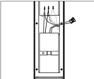
7. Remove the backing from adhesive tape on transformers, place in bottom of UPM body void of any wiring and press firmly for five seconds to ensure good contact.
