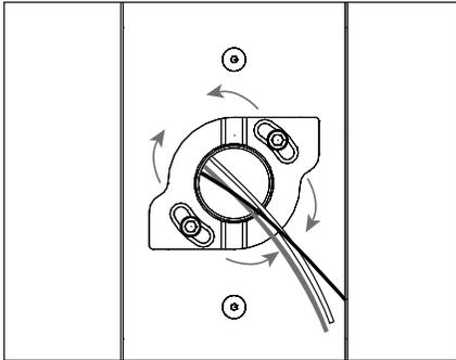
6. If UPM housing is not level, remove UPM housing; loosen but **DO NOT REMOVE** (2) #8-32 screws with 9/64" allen wrench on CamLock™ assembly. Adjust CamLock™ assembly up to 30° as needed to level. Tighten the screws and reattach UPM housing.
