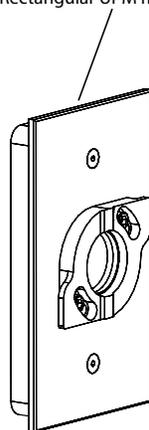
Patented 1/2" NPT knockouts\*
