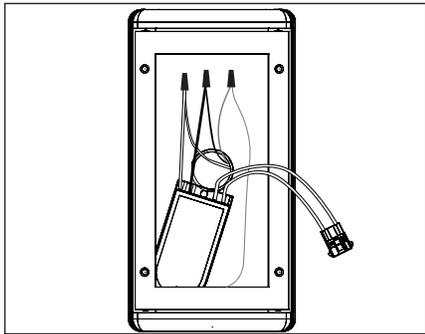
8. Remove the backing from adhesive tape on transformer, place in bottom of UPM housing void of any wiring and press firmly for five seconds to ensure good contact.
