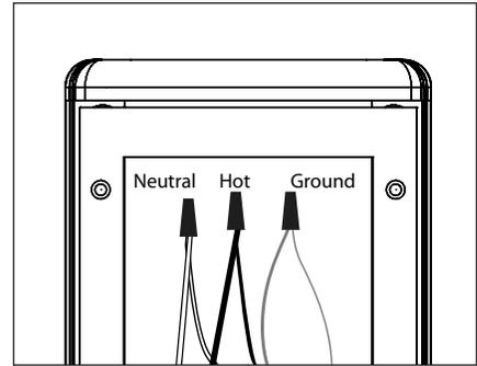
6. Use wire connectors (By Others) to connect transformer primary leads to branch circuit wires. Connect incoming ground to ground wire provided in UPM housing. See wiring diagram.
