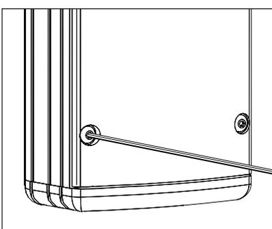
10. Make sure UPM body gasket is free of any dirt or debris. Attach the faceplate by tightening the (4) #6-32 captive screws evenly to 6-9 in/lbs using a 5/64" allen wrench.
