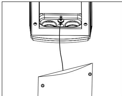
10. Attach tether wire under screw head at the base of the UPM housing. Slowly lower the faceplate until tether is taut.
