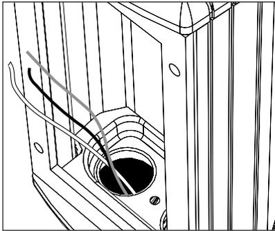
5. Pull branch circuit wiring necessary for installation (By Others.)
