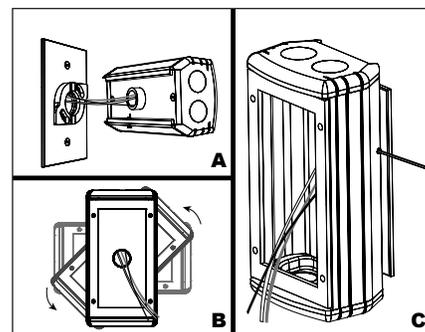
4. Feed wire into UPM housing. Install housing on CamLock™ at 90° to finished orientation as shown. (Figure A)
