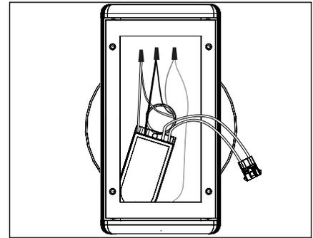
9. Remove the backing from adhesive tape on transformer, place in bottom of UPM housing void of any wiring and press firmly for five seconds to ensure good contact.
