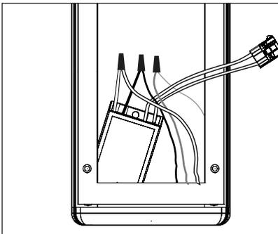
7. Remove the backing from adhesive tape on transformer, place in bottom of UPM body void of any wiring and press firmly for five seconds to ensure good contact.
