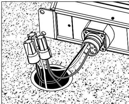
9. Use silicone filled wire nuts provided to connect branch circuit wiring to the anti-siphon (ASV™) wire pass-through located on the bottom of the UPM housing. See wiring diagram.
