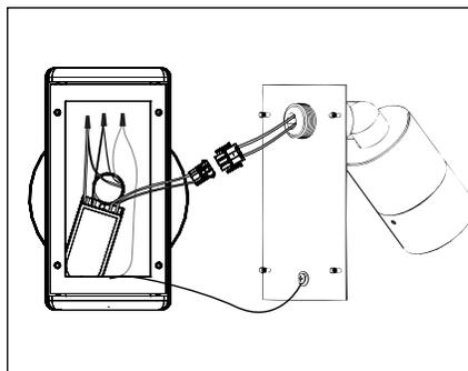
11. Connect transformer secondary leads to lamp leads using pre-wired factory connector.
