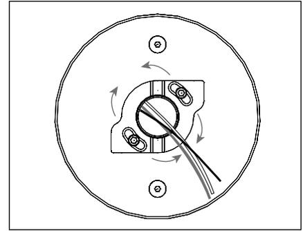
7. If UPM housing is not level, remove UPM housing; loosen but **DO NOT REMOVE** (2) #8-32 screws with 9/64" allen wrench on CamLock™ assembly. Adjust CamLock™ assembly up to 30° as needed to level. Tighten the screws and reattach UPM housing.
