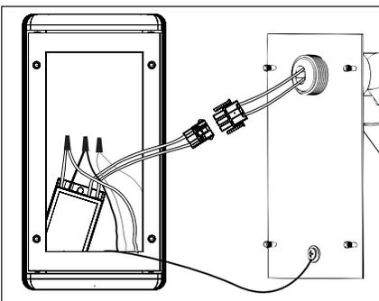
9. Connect transformer secondary leads to lamp leads using pre-wired factory connector.
