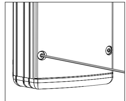
11. Make sure UPM body gasket is free of any dirt or debris. Attach the faceplate by tightening the (4) #6-32 captive screws evenly to 6-9 in/lbs using a 5/64" allen wrench.
