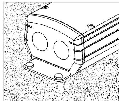
10. Anchor the UPM housing with mounting brackets provided using 1/4" fasteners (By Others).
