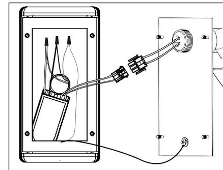
10. Connect transformer secondary leads to lamp leads using pre-wired factory connector.
