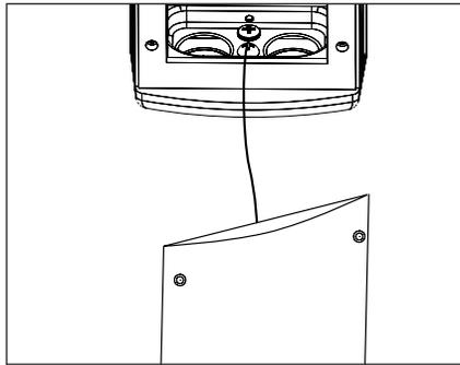
9. Attach tether wire under screw head at the base of the UPM housing and tighten. Slowly lower the faceplate until tether is taut.
