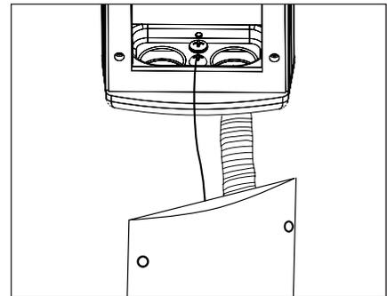
8. Attach tether wire under screw head at the base of the UPM housing and tighten. Slowly lower the faceplate until tether is taut.
