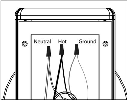
8. Use wire connectors (By Others) to connect transformer primary leads to branch circuit wires. Connect incoming ground to ground wire provided in UPM housing. See wiring diagram.
