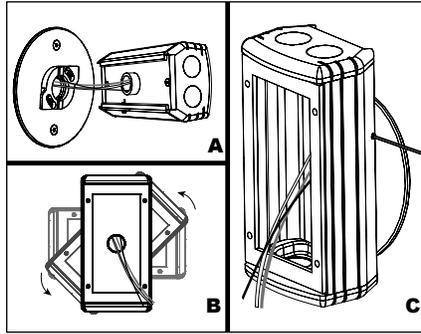
5. Feed branch circuit wiring into UPM housing. Install housing on CamLock™ at 90° to finished orientation as shown. (Figure A)
