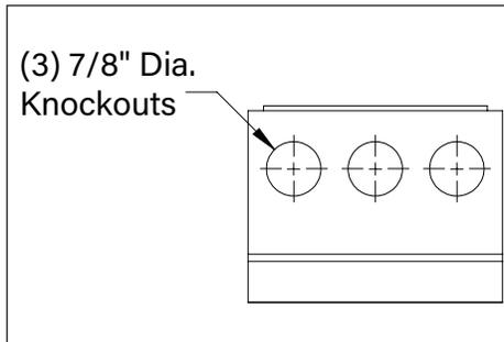
1. Mount transformer stainless steel housing with proper hardware for surface (hardware not included). Clearance holes are 4-1/4" apart on center.
