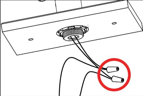
3. Make watertight connections from remote transformer to LED source leads using waterproof wire connectors. See wiring diagram.
