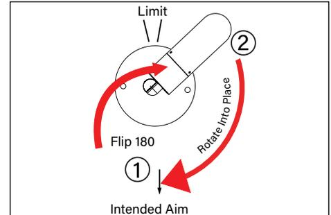
1. Use a 5/64" allen wrench to slightly loosen two (2) #8-32 set screw on the knuckle for 360° aiming purpose.
