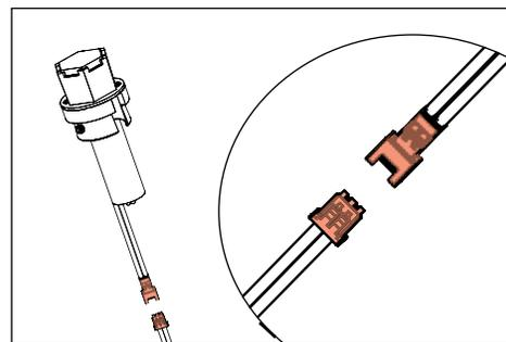
3. Disengage LED board and driver assembly. Replace with new board and driver assembly.
