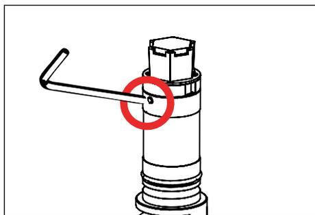
2. Use a .050" allen wrench to loosen two (2) #4-40 stainless steel set screws below LED board on the heat sink. Gently pull up on LED board and Driver assembly to expose quick disconnect.
