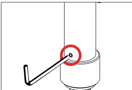
1. Use a 5/64" allen wrench to loosen #8-32 stainless steel set screw and remove cap.
