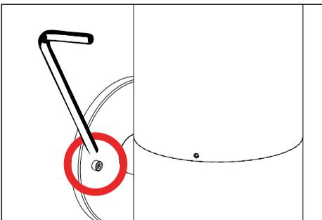
3. Mount fixture using two (2) #10-24 hex screws to installed back box using a 1/8" allen wrench. **Seal building envelope as per NEC. Do not overtighten.**
