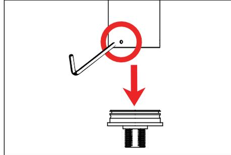
2. Use a 5/16" allen wrench to loosen three (3) #8-32 stainless steel set screws (**do not remove set screws from fixture**). Remove anchor base from the fixture.
