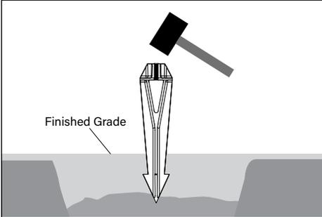
1. Drive the stake into the ground with a mallet or a small sledge hammer. Make sure the top is flush with the finished grade.
