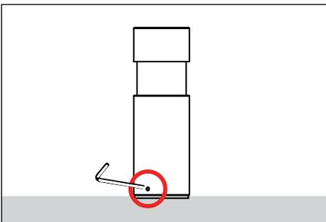
7. Install fixture onto anchor base. **Do not pinch wiring.** Secure fixture by tightening three (3) stainless steel set screws on fixture knuckle using a 5/64" allen wrench. **Do not overtighten set screws.**
