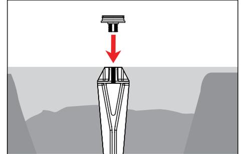
3. Attach the anchor base to the threads on the stake. Make sure the stake is secured in the ground.
