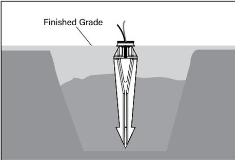
4. Pull low voltage, typically direct burial cable through the stake center where the hole is located to make the connect with the fixture.
