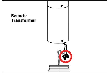
6. Make watertight connections from remote transformer to fixture leads using waterproof wire connectors (not included). **See wiring diagram.**
