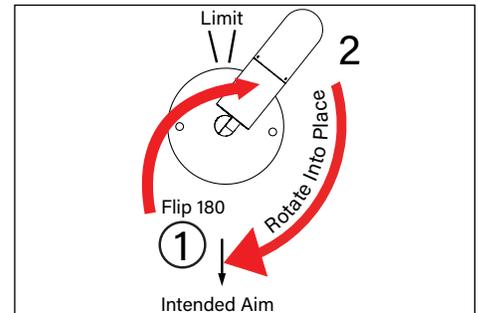
1. Use a 3/16" allen wrench to slightly loosen one (1) 3/8"-16 set screw on the knuckle for 360° aiming purpose.
