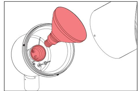
1. Loosen three (3) #10-32 stainless steel set screws on cap with a 5/32" allen wrench. Retain screws in cap.
