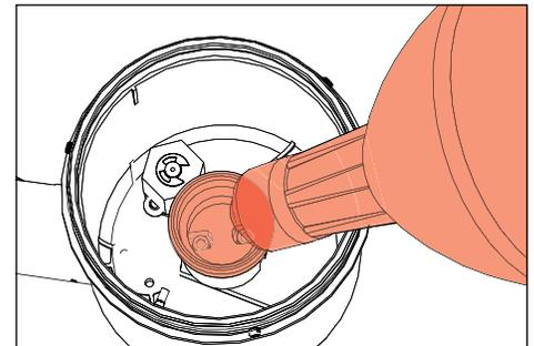
1. Loosen three (3) #10-32 stainless steel set screws with a 5/32" allen wrench on cap. Retain screws in cap.
