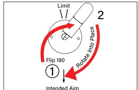
1. Use a 3/16" allen wrench to slightly loosen one (1) 3/8"-16 set screw on the knuckle for 360° aiming purpose.
