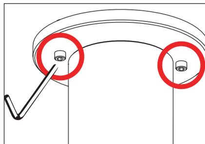
4. Mount fixture using two (2) #10-24 hex screws to installed back box. **Seal building envelope as per NEC. Do not overtighten.**
