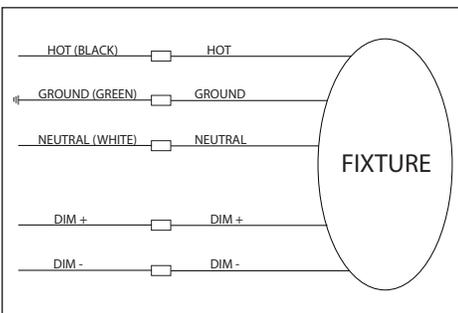
**WIRING DIAGRAM - Dimming 0/10**
