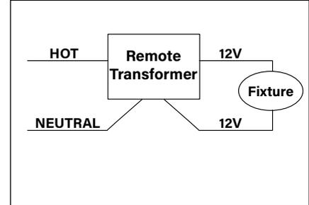
**WIRING DIAGRAM FOR USE WITH:**
