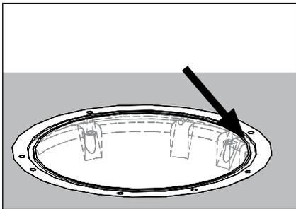
1. Before installation of faceplate, clean o-ring groove and collar of debris for a proper seal.
