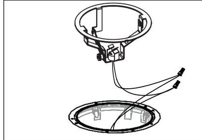
2. Make connections using silicone filled wire nuts (provided) from OptiLock to secondary wiring. See wiring diagram.
