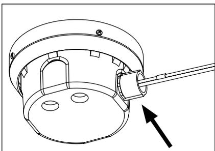
1. Secondary wiring is pre-wired with 5' leads. Pull 5' secondary leads from shallow HP2 housing through 3/4" conduit. Make watertight connections to secondary side of remote transformer using waterproof wire connectors in a waterproof splice compartment (not included) as per NEC.
