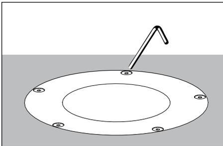
4. Install faceplate using a 1/8" allen wrench and hand-tighten the faceplate screws in a star pattern to 30 in-lbs. min.
