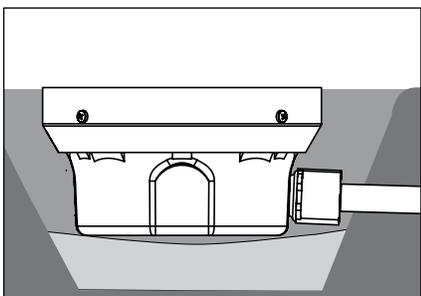
4. **For soil installation:** Fill and tamp soil to the appropriate height leaving room for sod, pavers, etc. to be level with the top of the faceplate.
