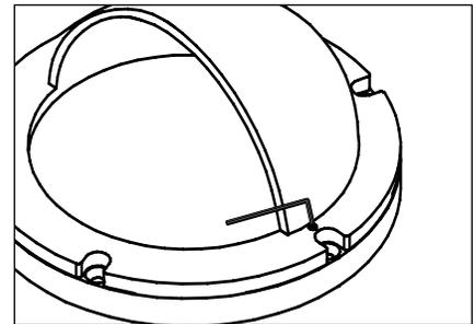
3. Using a 7/64" allen wrench, loosen the two (2) #6-32 set screws on the faceplate to allow accessory to rotate freely.
