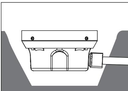
2. Place housing in excavated hole. Align power cord with leads in the path of the conduit trench(es).
