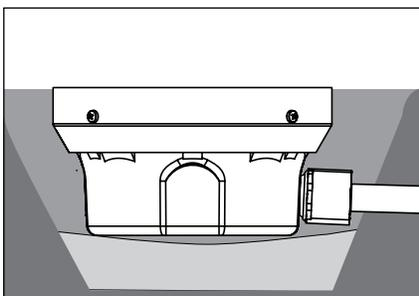
5. **For concrete installation:** Fill the hole around the fixture housing to 12" below the finished grade with clean fill dirt and tamp carefully to prevent settling of fixture. Pour concrete and finish as required flush with the top surface of the temporary cover.
