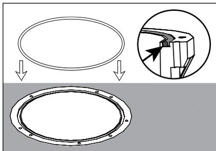
7. Remove any dirt or debris in o-ring groove near top of housing. Place o-ring inside of groove.
