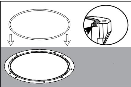
3. Remove any dirt or debris in o-ring groove near top of housing. Place o-ring inside of groove.
