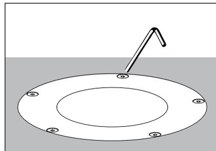
8. Install faceplate using a 1/8" allen wrench and hand-tighten the faceplate screws in a star pattern to 30 in-lbs. min.
