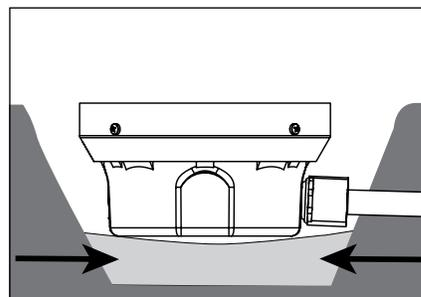
3. Per DIG-IT Guide, backfill the gap between the bottom of housing and bottom of hole with sand for drainage.
