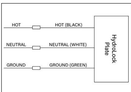
**WIRING DIAGRAM FOR USE WITH:**
