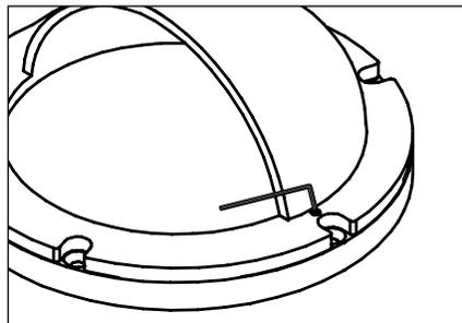
5. When set in final position, tighten two (2) #6-32 set screws using a 7/64" allen wrench.
