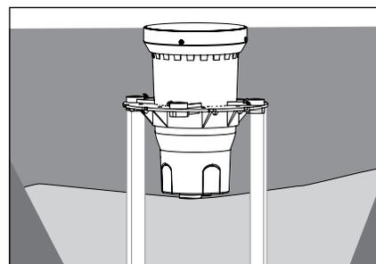
7. Per DIG-IT Guide, backfill the gap between the bottom of housing and bottom of hole with sand for drainage.
