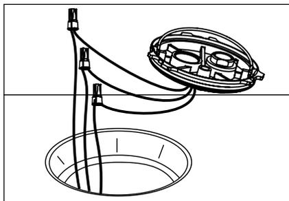
2. Make watertight connections using waterproof wire connectors (provided) to leads on the bottom of Patented HydroLock Barrier Plate Assembly. **See wiring diagram.**
