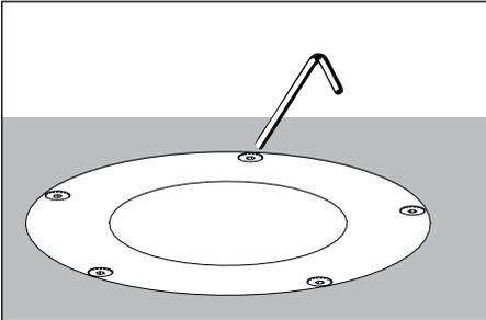
1. Remove faceplate using a 1/8" allen wrench. If there is an optional accessory holder, carefully squeeze tabs on sides and gently pull from slots on OptiLock.
