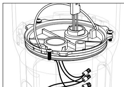
4. Turn HydroLock Barrier Plate clockwise ¼" to lock.
