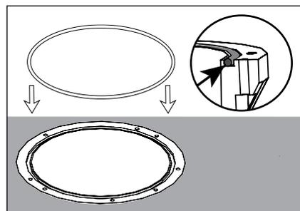
10. Remove any dirt or debris in o-ring groove near top of housing. Place o-ring inside of groove.
