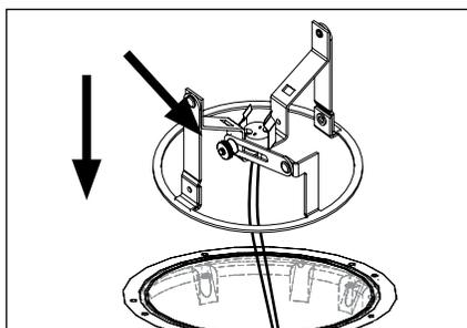
6. Place OptiLock in HP2 housing and align keyhole notch under one of three (3) #8 screw heads. Rotate horizontally to desired aiming position, then tighten two (2) #8 Phillips screws using Phillips screwdriver. Install proper MR16 halogen, PAR36/AR111, PAR20/30, or GU10 lamp according to instructions on Lamp Installation Or Re-Lamping page.
