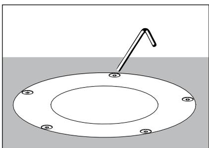
11. Install faceplate using a 1/8" allen wrench and hand-tighten the faceplate screws in a star pattern to 30 in-lbs. min.
