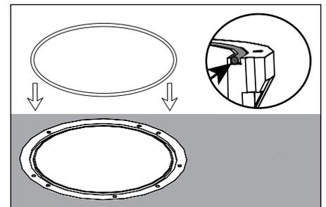
3. Remove any dirt or debris in o-ring groove near top of housing. Place o-ring inside of groove.
