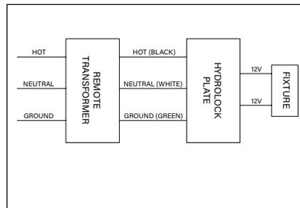
**WIRING DIAGRAM FOR USE WITH:**
