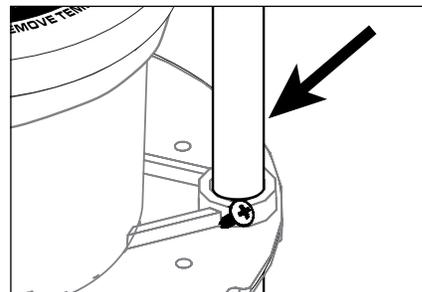
1. Connect branch conduit connectors (not included) to the junction box using either the threaded conduit entries on the bottom of the junction box or through holes drilled into the sides of the junction box.
