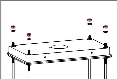
1. Remove 1/4-20 nuts from installed YKB anchor kit with a socket. Keep the hardware to reuse in the next step.
