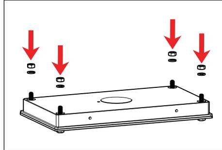
2. Line up then place base over installed 1/4-20 nuts.
