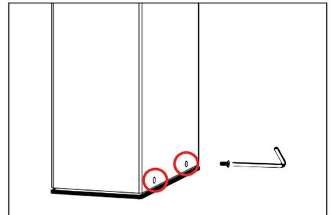
6. Attach receptacle to installed anchor base with four (4) #10-32 stainless steel countersunk screws at the base using a 1/8" allen wrench.
