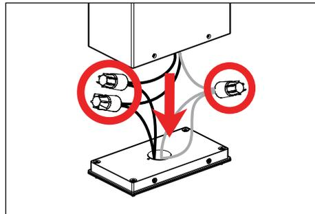
5. Pull primary branch circuit wiring and any additional dimming controls or other wiring necessary for installation. Attach ground from branch circuit to ground lead on the anchor base. Place connectors inside of the housing (**Please refer to page 4 for wiring diagram**).
