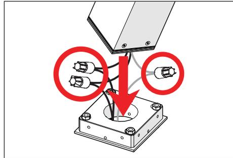
5. Pull primary branch circuit wiring and any additional dimming controls or other wiring necessary for installation. Place connectors inside of the housing (Please refer to page 4 for wiring diagram).
