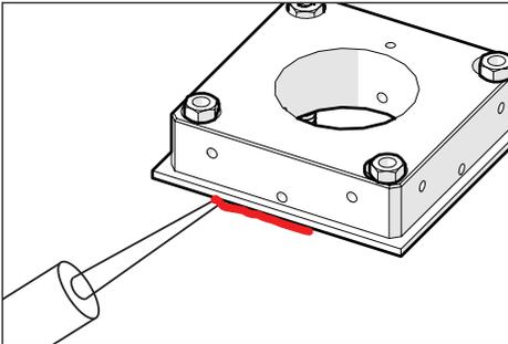
4. Seal as per NEC with waterproof silicone sealant (not included).
