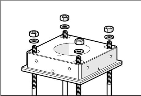
1. Remove 1/4-20 nuts from installed Union anchor kit with a socket. Keep the hardware to reuse in the next step.
