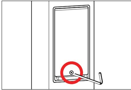
7. Receptacle cover has captive #6-32 screw. Secure receptacle by tightening captive #6-32 set screw using a 7/64" allen wrench.
