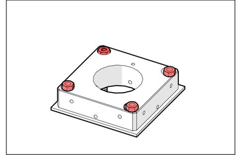
3. Secure to anchor bolts with the 1/4-20 nuts and lockwashers provided with the Union anchor kit using a socket.
