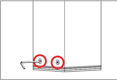
6. Attach in-use receptacle to installed anchor base and plate with four (4) #10-32 stainless steel cap screws at the base using a 1/8" allen wrench.
