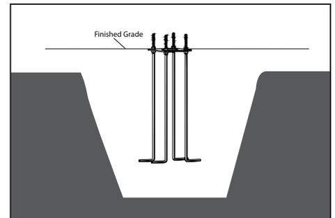
1. Adjusted anchor bolts to project at least 1-1/2" using the four (4) 1/4-20 nuts to the top of the plate. The four (4) nuts can be left in place while concrete is poured.
