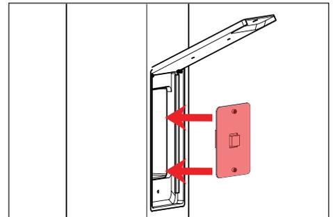
1. Open receptacle cover. Receptacle cover has #6-32 screw for use with a 7/64" allen wrench.
