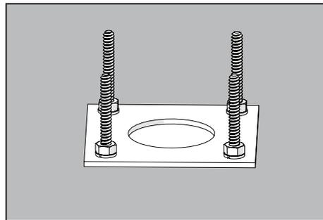
4. With the conduits in place and the anchor plate properly positioned, secured and leveled, concrete may be poured.
