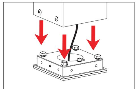
4. Place connections into bollard. Attach inner bracket with RJ45 jack with two (2) #6-32 screws with a 7/64" allen wrench.
