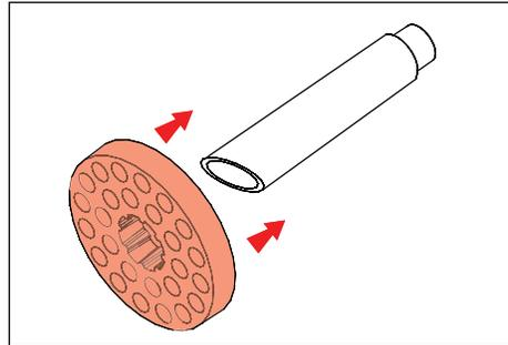
2. Slide optional Stability Flange onto Power Pipe. Use optional Stability Flange to aid in installation of power pipe.
