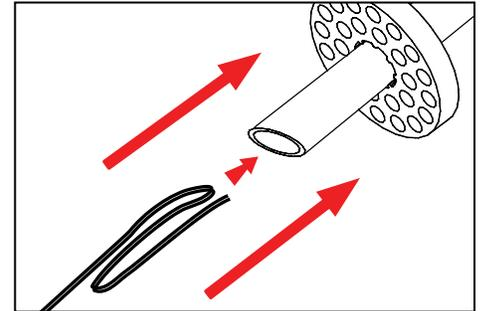
3. Pull low voltage wiring from remote transformer to power pipe. Allow for additional cable to make connections to fixture lead and future service.
