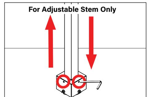
4. Slide stem up or down to desired height. Delrin bushing holds stem in position. Tighten the four (4) #10 stainless steel set screws using a 3/32" allen wrench to lock mounting height in place. Unused stem length remains hidden inside power pipe to accommodate future landscape growth.
