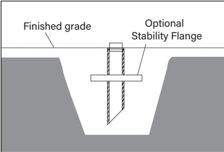
1. Excavate trench according to designed lighting plan. Dig hole a minimum of 24" deep and 10" wide to accommodate power pipe at desired fixture locations.
