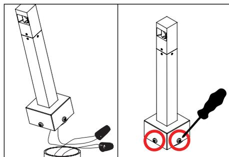
2. Insert additional wires and connectors into power pipe. Place fixture on power pipe.
