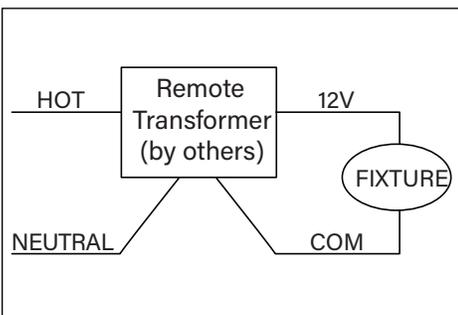
1. Make watertight connections from remote 12V transformer to fixture leads using waterproof wire connectors (not included).
