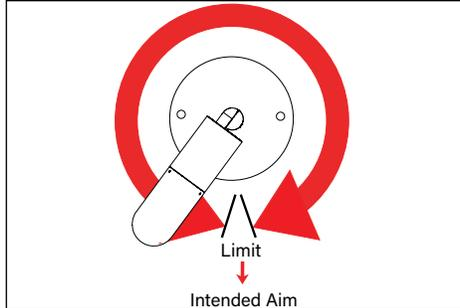
3. If the over-rotation protection pin is in the desired aiming position, do not force the fixture past the limit. Using a 3/16" allen wrench, slightly loosen both set screws in the knuckle, enough to move the fixture freely on both axes.
