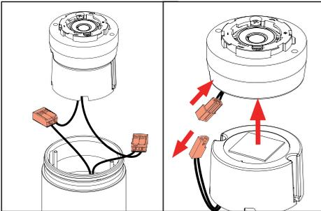
4. Disconnect driver assembly from fixture body.
