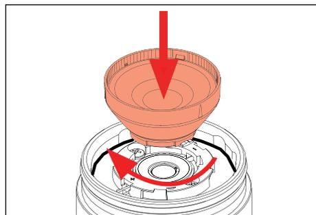
10. Twist to reinstall optic onto optic holder.
