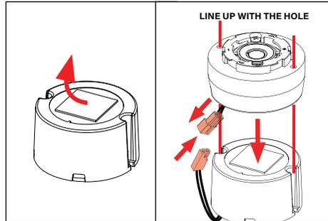
6. Remove protective plastic from the double-sided tape square on clean top of driver assembly.
