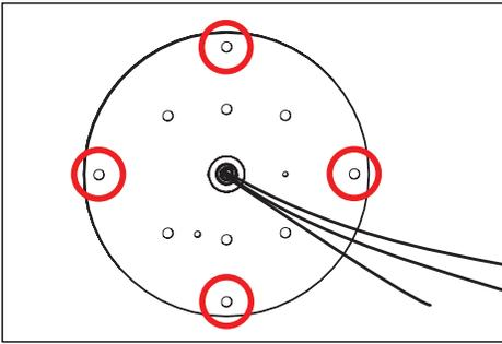
4. Circled locations are mounting holes for mounting heavy duty mounting plate to substrate. Use mounting hardware (hardware not included) suitable for substrate material. **Seal building envelope as per NEC.**
