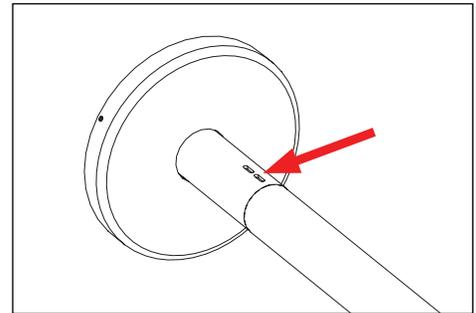
8. Tighten set screw when cable notch in stem is in line with support cable and support canopy.
