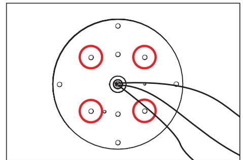
1. Pull fixture leads through heavy duty mounting plate. Make watertight connections from remote driver to fixture leads using waterproof wire connectors (not included). **See wiring diagram**.
