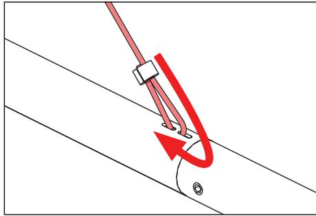
10. Thread aircraft support cable through cable notch in stem. Loop and fasten with compression fitting. Use proper crimping tool to close compression fitting.
