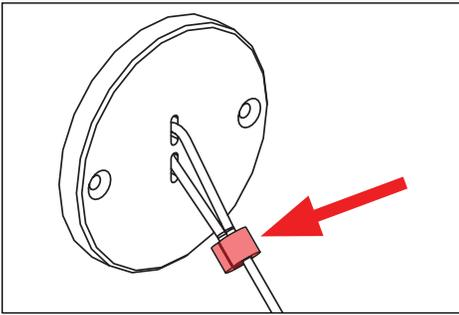
9. Thread aircraft support cable through support canopy cable notch. Loop and fasten with compression fitting. Use proper crimping tool to close compression fitting.
