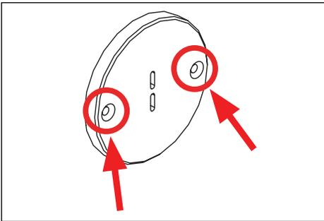
6. Mount support canopy above fixture location using appropriate mounting hardware for surface. **Seal building envelope as per NEC. Do not overtighten.**
