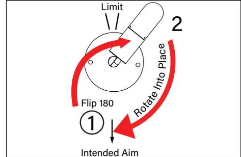
4. Flip the fixture 180 degrees over the knuckle. The rotational range limit will now be 180 degrees from the original position. Now rotate the fixture into the desired aiming position.
