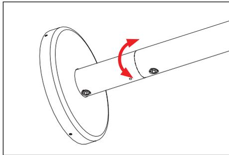
7. Adjust stem so that cable notch in stem lines up with support canopy location and cable. Loosen 3/8" set screw in stem to adjust.
