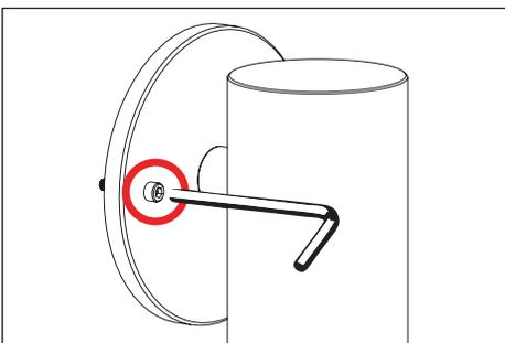
4. Mount fixture using two (2) #10-24 hex screws to installed back box. **Seal building envelope as per NEC. Do not overtighten.**
