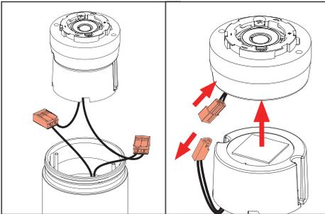
4. Disconnect driver assembly from fixture body.
