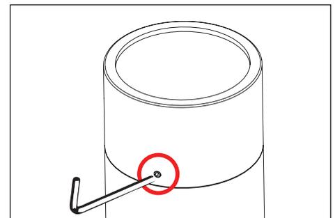
11. Install cap by tightening three (3) #8-32 set screws with a 5/64" allen wrench. **Do not over tighten.** Cap should be able to rotate without force.
