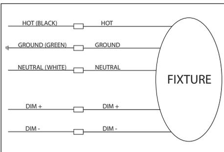
**WIRING DIAGRAM - Dimming**
