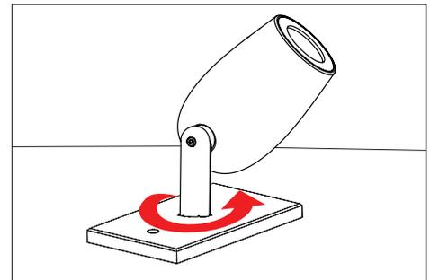
6. Rotate fixture at base and aim fixture to desired horizontal location.
