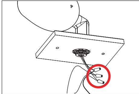
3. Make watertight connections from remote transformer to fixture leads using waterproof wire connectors (not included). **See wiring diagram.**
