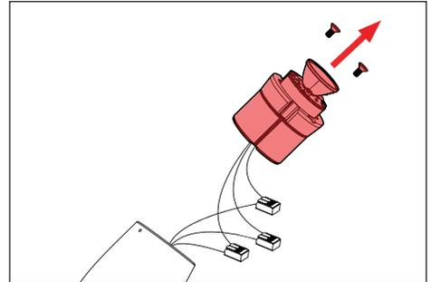
3. Disengage laser board and driver assembly.
