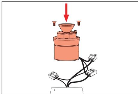
5. Connect new driver assembly to fixture leads. Place connections inside body cavity, reinsert new heatsink assy back into body. Reinstall two (2) 8-32 flat head cap screws completely onto the heatsink until screws catch under the groove on the body. Rotate the two (2) 8-32 flat head cap screws counterclockwise until they are snug against the top of the groove.
