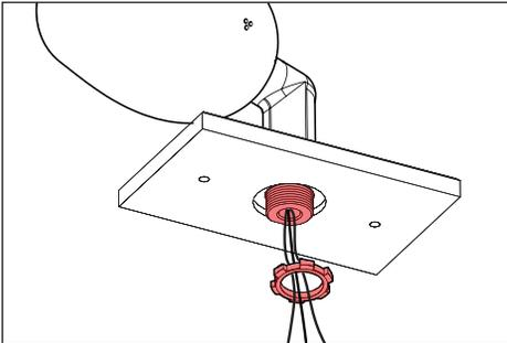
1. Mount knuckle onto suitable enclosure according to designed lighting plan.
