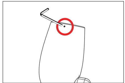
6. Place cap on fixture and tighten set screw. Tighten screw to 1/2 in-lbs. Top of screw should sit flush with fixture body.
