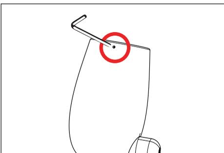
1. Use a 1/16" allen wrench to loosen #6-32 stainless set screw and remove cap.
