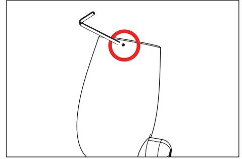
6. Place cap on fixture and tighten set screw. Tighten screw to 1/2 inch pounds. Top of screw should sit flush with fixture body.
