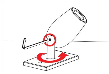
4. Use a 5/32" allen wrench to slightly loosen #10-32 stainless steel black oxide socket head cap screw at the knuckle for aiming purposes. Tighten to secure desired location.
