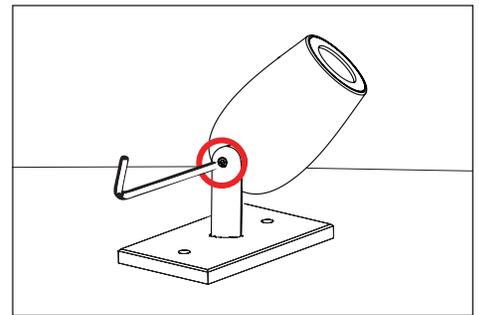
3. Use a 5/32" allen wrench to loosen #10-32 stainless steel black oxide socket head cap screw at the knuckle for vertical aiming purpose.
