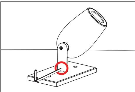
1. Use A 5/64" allen wrench to slightly loosen two (2) #8-32 stainless steel set screws on the stem for 360° aiming purpose.
