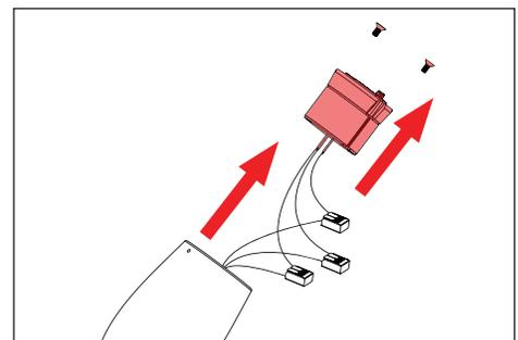
3. Disengage LED board and driver assembly.
