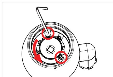
2. Rotate the two (2) 8-32 flat head cap screws using a 3/32" allen wrench clockwise until they bottom out into the heatsink, then rotate the heatsink so the screws line up with the grooves. Remove the two (2) 8-32 flat head cap screws from the heatsink completely.
