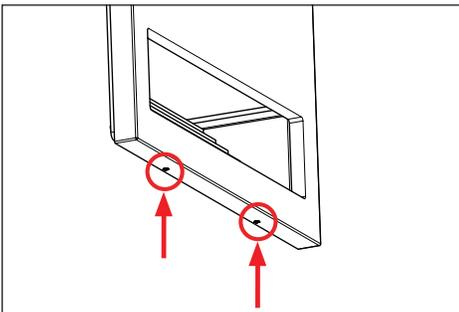
10. Then lower bottom side of faceplate onto fixture. Secure by tightening two (2) #6-32 set screws using a 1/16" allen wrench. **Do not overtighten.**
