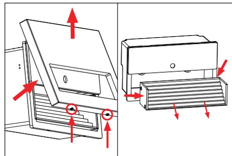
3. Prepare fixture for installation. Remove faceplate from housing by loosening two (2) #6-32 set screws using a 1/16" allen wrench. **Do not fully remove set screws.**
