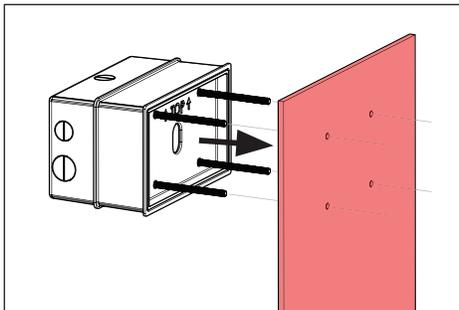
5. Install housing and sleeve assembly onto concrete form. Pass all threads through mounting holes.
