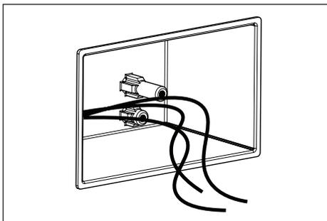
2. Remove installation sleeve. Pull primary branch circuit wiring and/ or dimming control wiring necessary for installation.
