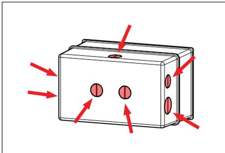
2. Housing is provided with six (6) 1/2" and two (2) 3/4" conduit entries. Knockout or drill out using a hole saw on desired conduit entry point. Install conduit onto housing.
