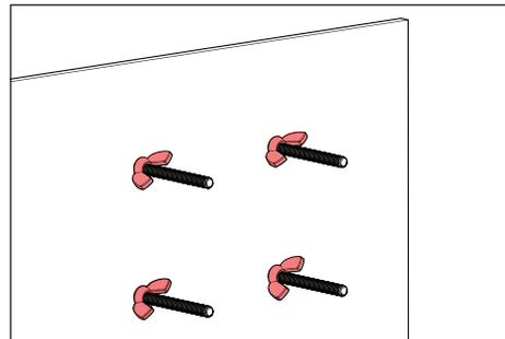
6. Hand tighten four (4) wingnuts onto all threads until housing assembly is firmly secured against the inside face of concrete form.
