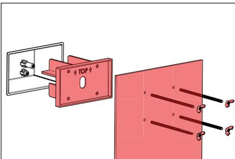
1. Once concrete is cured, remove concrete form and all threads from housing. Leave installation sleeve inside housing until fixture is ready to be installed to prevent debris from building up in housing.
