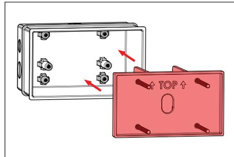
3. Reinstall installation sleeve into housing. Inscription "TOP" on sleeve indicates top side of fixture for correct fixture orientation.
