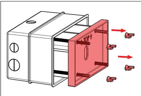
1. Prepare housing for installation. Remove installation sleeve by removing four (4) wing nuts. Set aside for later use.
