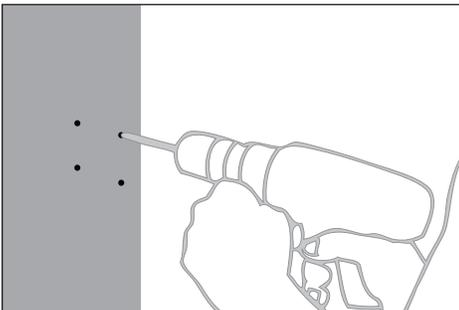
4. Drill four (4) 1/4" holes at desired position on concrete form. Mounting against a flat surface like a plywood form is recommended. Use provided mounting hole template on pg 4.
