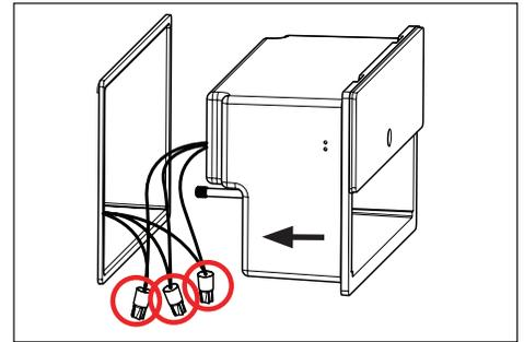
5. Make watertight connections from line voltage to fixture leads using waterproof wire connectors.
