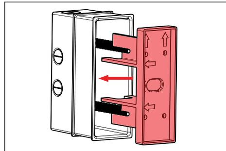
3. Insert plastic sleeve into housing previously removed on step 1.
