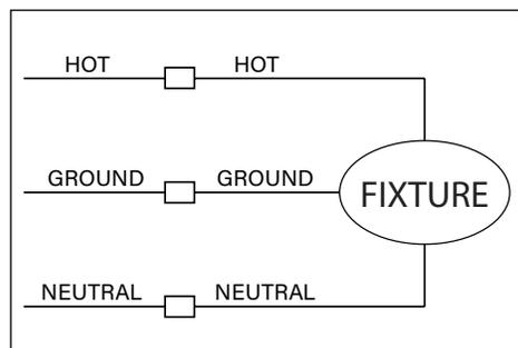
4. Make watertight connections from line voltage to fixture leads using waterproof wire connectors.
