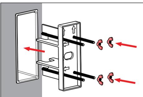
1. Remove plastic sleeve and all-threads by removing wing nuts.
