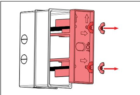
1. Remove 4 wing nuts and plastic sleeve from housing and save for later use.
