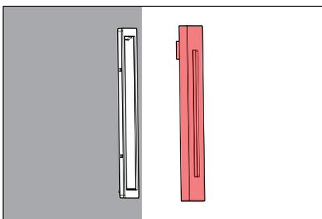
2. Remove faceplate from fixture by lifting from the bottom up and save for later use.
