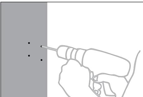
4. Drill four 1/4" holes at desired position on concrete form. Please use 1-1 template provided on page 4.
