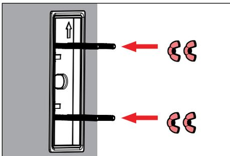
5. Insert all-threads through the four 1/4" holes drilled on the concrete form and install in to the housing. Then hand tighten the 4 wing nuts previously removed in step 1.
