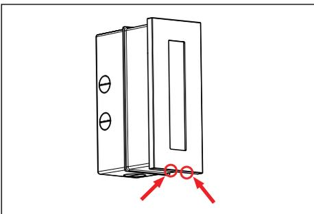
1. Tighten two #8-32 stainless steel set screws at the bottom of the faceplate with a 5/64" allen wrench.
