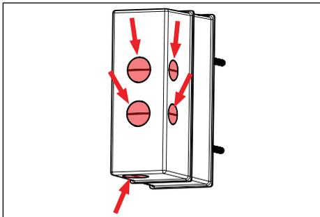
2. Knock out one of the knockouts on the back or side of the housing and install conduit.
