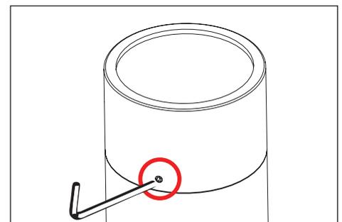
10. Install the cap on by tightening three (3) #8-32 set screws by using a 5/64" allen wrench. **Do not over tighten. Cap should be able to rotate without force.**
