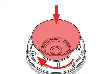
9. Twist to reinstall optic onto optic holder.
