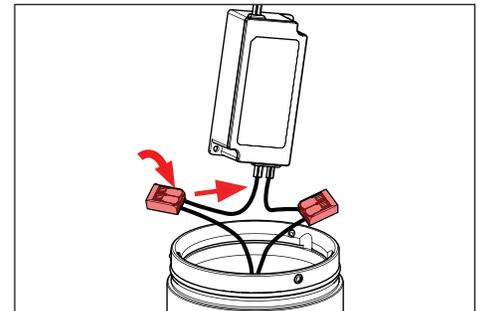
7. Reconnect heatsink assembly to driver assembly via quick disconnect. Quick disconnect tucks into space underneath heatsink.
