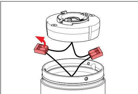
4. Lift lever on the wago connector to remove LED leads.
