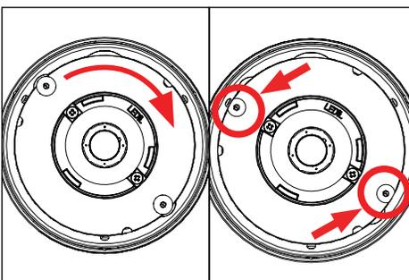
8. Align the flat head screws with slots in the fixture and reinstall the heatsink back on. Rotate the heatsink into place and loosen the two (2) #8-32 flat head screws using a 3/32" allen wrench to engage heatsink.
