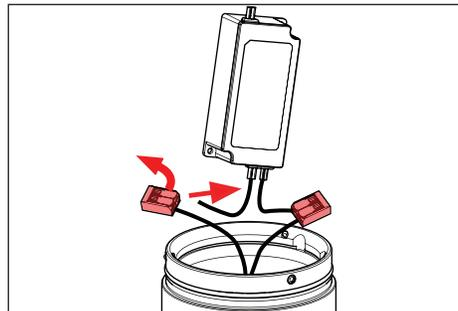
6. Remove driver from fixture via quick disconnect. Replace with the new driver and reinstall into fixture.
