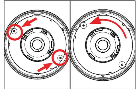
3. Disengage the heatsink by tightening the two (2) #8-32 flat head screws by using a 3/32" allen wrench. Rotate the heatsink to align the screws with slots to remove.
