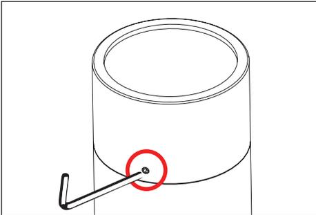
1. Loosen three (3) #8-32 set screws on the cap by using a 5/64" allen wrench. Do not remove set screws, firmly pull on the cap to remove.
