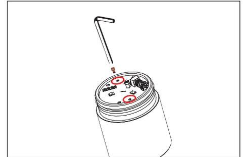
3. Use a 5/64" allen wrench to remove two (2) #2-56 socket head cap screws on LED board, grasp LED board and gently pull up to expose quick disconnect.
