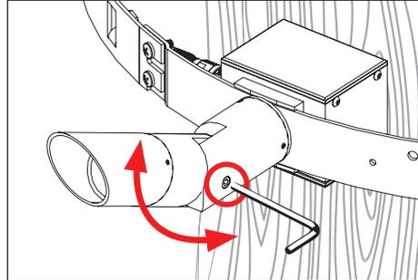
1. Use a 5/64" allen wrench to loosen three (3) #8-32 stainless steel set screws on fixture base. Rotate fixture at base and aim fixture to desired horizontal location, then tighten screw.
