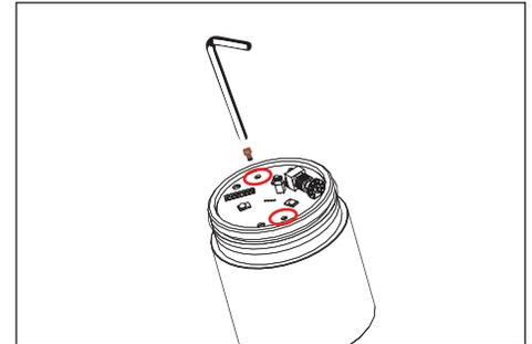
1. Use a 5/64" allen wrench to loosen #8-32 stainless set screw and remove cap.
