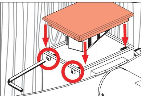
7. Replace top of transformer housing with four (4) #8-32 screws with a 5/64" allen wrench.
