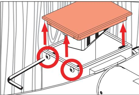
4. Remove top of transformer housing by removing four (4) #8-32 set screws using a 5/64" allen wrench.
