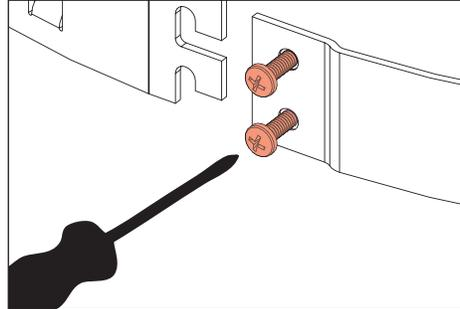
2. Secure by hooking end of strap over two (2) phillips screws. Secure by tightening two (2) phillips screws with phillips screwdriver.
