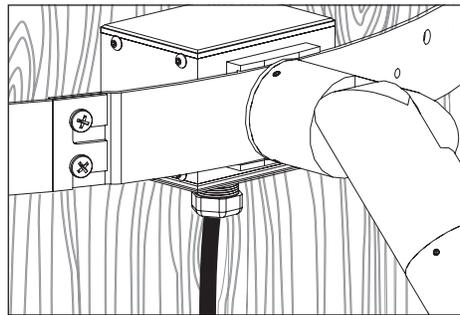
5. Bring line voltage cable from power line to main splice box location. Loosen cord grip on bottom of splice box, feed linevoltage cable from power line through, then tighten cord grip to secure.
