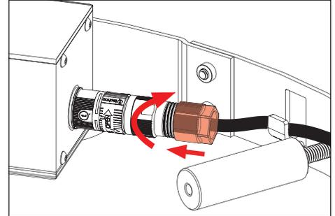
3. Connect secondary cable then twist to secure in place.
