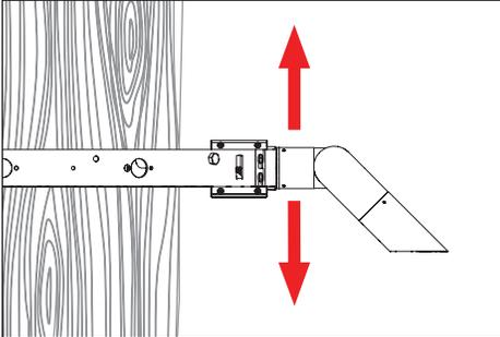
1. Place tree ring fixture around tree. Move fixture to desired height. Tighten the entire assembly to the tree with provided stand-offs.
