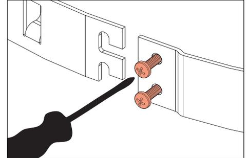
4. Secure by hooking end of strap over two (2) phillips screws. Secure by tightening two (2) phillips screws with phillips screwdriver.
