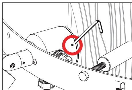
7. Close main splice box with three (3) #8-32 set screws using a 5/64" allen wrench. Secondary side of fixture and additional fixtures are factory pre-wired. Adjust fixture aiming as required.
