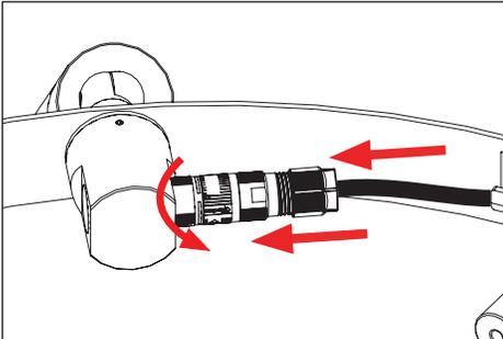
5. Connect secondary cable then twist to secure in place.
