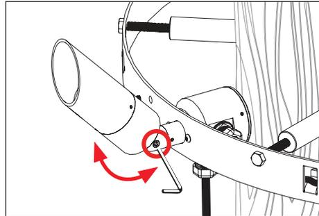
2. Use a 5/32" allen wrench to loosen #10-32 stainless steel black oxide socket head cap screw at the knuckle for vertical aiming purpose, then tighten screws.
