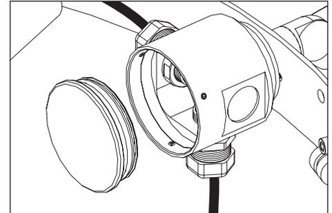
5. Bring low voltage cable from remote transformer secondary side to main splice box location. Loosen cord grip on bottom of splice box, feed low voltage cable from remote transformer through, then tighten cord grip to secure.
