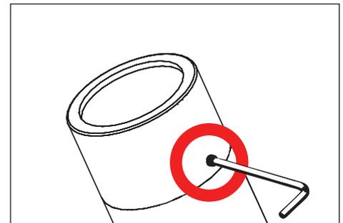
6. With flat head screw driver rotate dial to desired lumen output. Replace cap.
