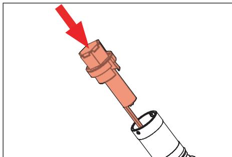
4. Reverse install LED board and driver by carefully wrapping 18 gauge wires around driver and inserting into fixture body. Secure LED board in place with two (2) #4-40 stainless steel set screws.
