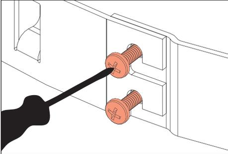
1. Locate side of strap without factory pre-wired cable. To open strap, use Phillips screwdriver to back out strap screws. Strap hooks over two (2) phillips screws on strap.
