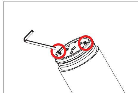
3. Use a 5/64" allen wrench to remove two (2) #2-56 socket head cap screws on LED board, grasp LED board and gently pull up to expose quick disconnect.
