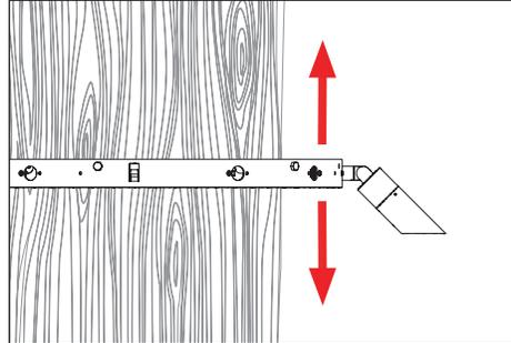
3. Place tree ring fixture around tree. Move fixture to desired height. Tighten the entire assembly to the tree with provided stand-offs.
