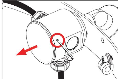
6. Open main splice box by loosening three (3) #8-32 set screws using a 5/64" allen wrench. Main splice box has cord grip on bottom of splice box.
