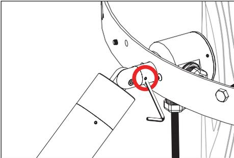
1. Use a 5/64" allen wrench to slightly loosen two (2) #8-32 stainless steel set screws on the stem for 360° aiming purpose, then tighten screws.
