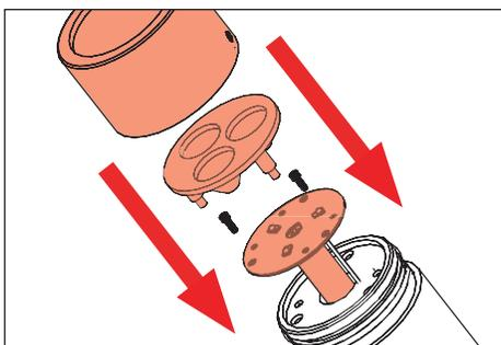
5. Reverse install LED board and driver by carefully wrapping 18 gauge wires around driver and inserting into fixture body. Secure LED board in place with stainless steel screws.
