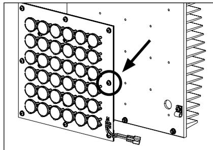
4. **If replacing LED board:** Remove LED board and thermal pad from heatsink by loosening sixteen (16) Phillips screws using Phillips screwdriver. Line up new thermal pad and LED board on heatsink. Replace board and thermal pad on heatsink with thermal pad closest to heatsink, then reverse install.
