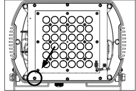
2. Prepare to remove LED board, thermal pad and heatsink by loosening six (6) #8-32 slotted screws using a 1/4 nut driver/socket wrench or a flat head screwdriver.
