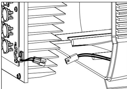
7. Reconnect quick disconnect from driver secondary side to LED board assembly.
