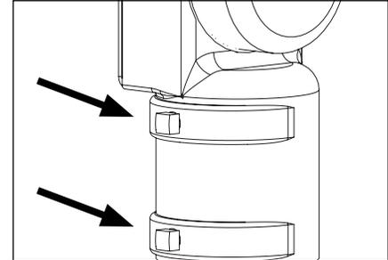
1. Install pole with standard 2" tenon mount (2-3/8" outer diameter) according to manufacturer's instructions (pole not included). Pull incoming primary branch circuit wiring.
