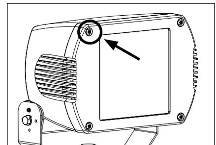
9. Replace faceplate by tightening four (4) tamper-resistant hex screws using a Torx T27 tamper resistant hex bit.
