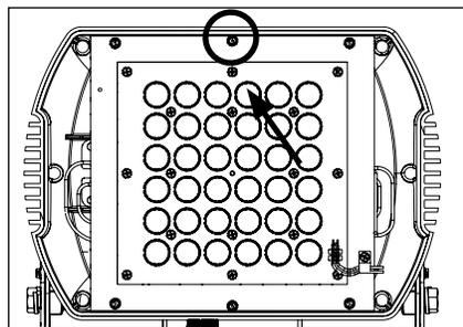
8. Secure LED board and heatsink by tightening six (6) #8-32 slotted screws using a 1/4 nut driver/socket wrench or flat head screw driver.
