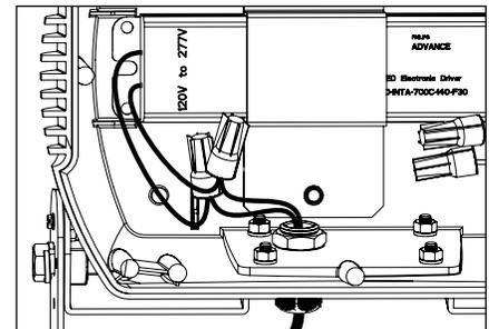
5. **If replacing LED driver:** Turn off branch circuit. Disconnect wire nuts from incoming primary to primary side of driver.
