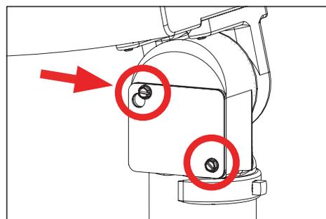
4. Fit fixture over pole tenon and ensure it is completely seated. Secure fixture to tenon by tightening two (2) 3/8"x16 stainless steel square screws using an adjustable crescent wrench.
