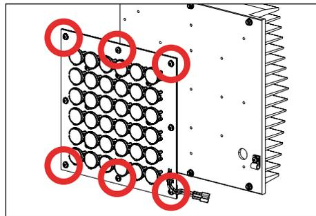
4. **If replacing LED board:** Remove LED board and thermal pad from heatsink by loosening sixteen (16) Phillips screws using Phillips screwdriver. Line up new thermal pad and LED board on heatsink. Replace board and thermal pad on heatsink with thermal pad closest to heatsink, then reverse install.
