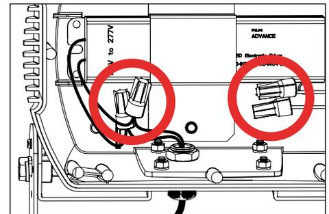
5. **If replacing LED driver:** Turn off branch circuit. Disconnect wire nuts from incoming primary to primary side of driver.
