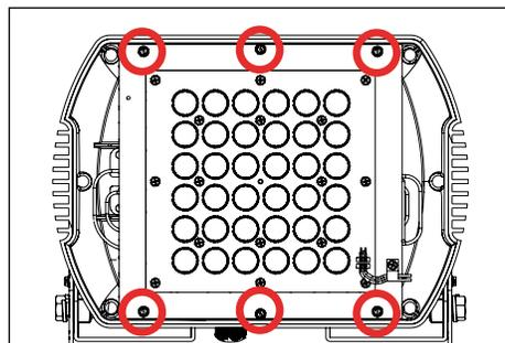
8. Secure LED board and heatsink by tightening six (6) #8-32 slotted screws using a 1/4 nut driver/socket wrench or flat head screw driver.
