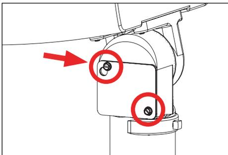
7. Attach wiring compartment access panel to knuckle wiring compartment by tightening two (2) screws using 5/16" socket wrench.
