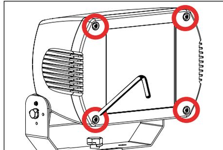
1. Remove faceplate by loosening four (4) tamper-resistant hex screws using a Torx T27 tamper resistant hex bit.
