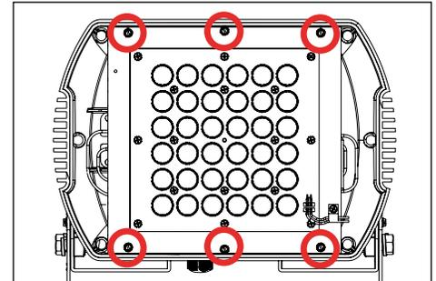
2. Prepare to remove LED board, thermal pad and heatsink by loosening six (6) #8-32 slotted screws using a 1/4 nut driver/socket wrench or a flat head screwdriver.
