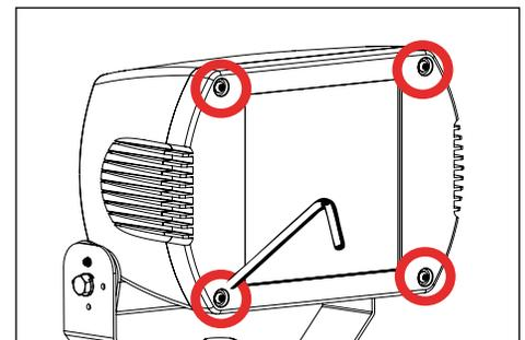
9. Replace faceplate by tightening four (4) tamper-resistant hex screws using a Torx T27 tamper resistant hex bit.
