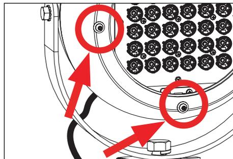
7. Place connections inside wiring compartment in slipfitter. Close panel to wiring compartment in slipfitter by tightening four (4) #10-24 hex washer heads using adjustable crescent wrench, 8mm socket wrench, or flat head screwdriver.
