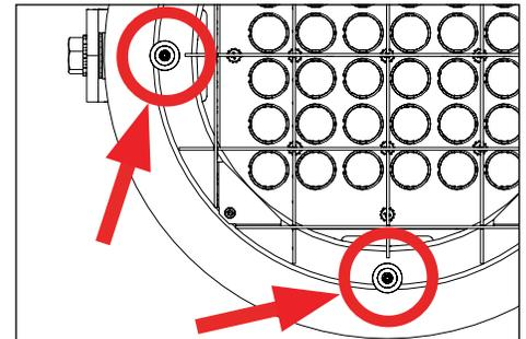
6. To relamp: remove faceplate and louver by loosening four (4) tamper resistant screws using a TORX T27 socket (1/4" bit). Relamp as needed, then reverse install.
