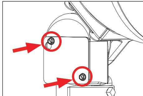
5. Attach wiring compartment access panel to knuckle wiring compartment by tightening two (2) screws using a 5/16" socket wrench.
