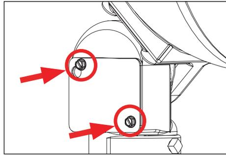
2. Remove wiring compartment access panel to knuckle wiring compartment by loosening two (2) screws using a 5/16" socket wrench.
