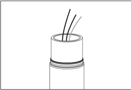
1. Pull branch circuit wiring needed, through pole tenon.
