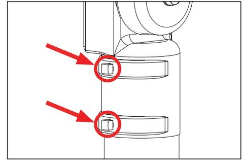
3. Fit fixture over pole on mounting plate and ensure it is completely seated. Secure fixture to pole by tightening two (2) 3/8"x16 stainless steel square screws using an adjustable crescent wrench.
